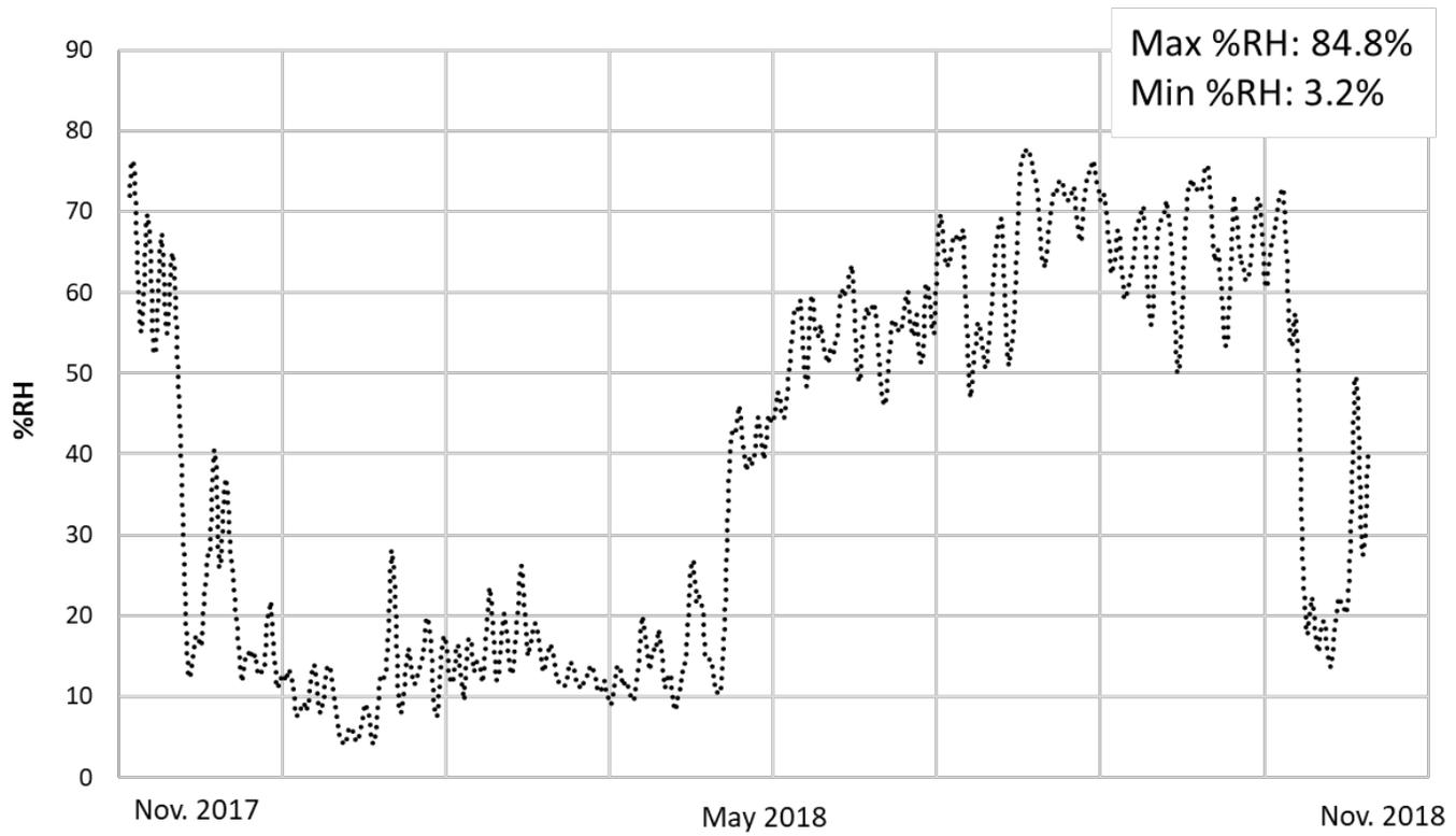
**Figure 5:** Percent Relative Humidity (% RH) from November 2017 – November 2018 for two data loggers stored at Facility Seven. Data is plotted as a 50-point moving average for visualization purposes. Maximum and minimum temperatures reported are noted for each data logger.
