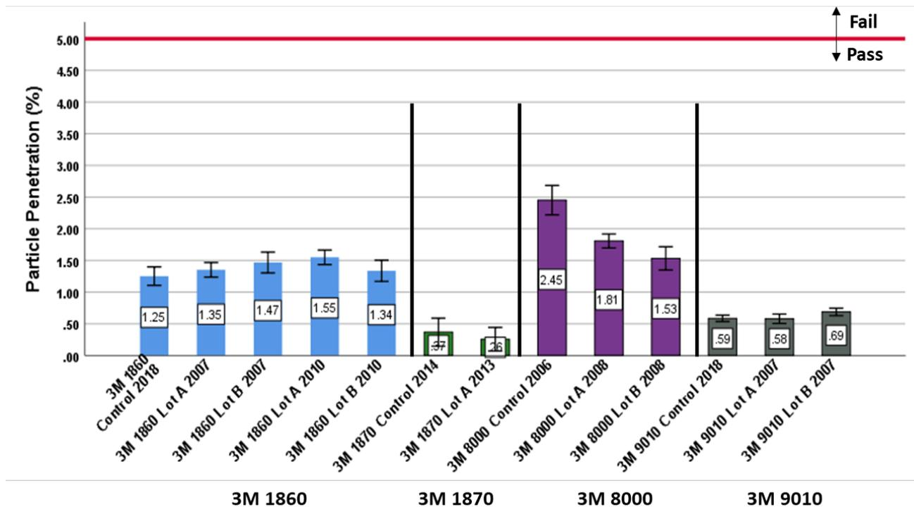
**Figure 9:** Control and stockpiled respirator particle filtration performance data for the 3M 1860, 3M 1870, 3M 8000, and 3M 9010 models. N95 FFRs must have a particle penetration of less than 5.0%. Error bars represent the 99% confidence interval and estimate the population parameters. This confidence interval suggests that 99% of any repeated samples tested and evaluated from this lot will have a mean between the upper and lower bounds.
