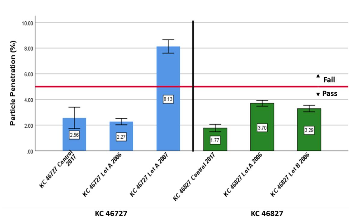
**Figure 12:** Control and stockpiled respirator particle filtration performance data for the KC 46727 and KC 46827 models. N95 FFRs must have a particle penetration of less than 5.0%. Error bars represent the 99% confidence interval and estimate the population parameters. This confidence interval suggests that 99% of any repeated samples tested and evaluated from this lot will have a mean between the upper and lower bounds.
