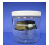
Permeation Test Vessel
