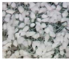
Textile Swatch Containing NanoActive Aluminum Oxide Plus
