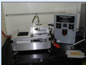
Fig 1. Stored Thermal Energy Test Apparatus
