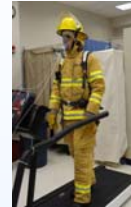
Figure 2. Subject during a comparison session, wearing standard firefighter ensemble over LifeShirt.
