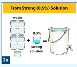
Pour 9 parts water and 1 part strong (0.5%) solution into a bucket. Repeat until full.
