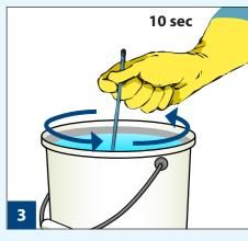
Stir well for 10 seconds, or until the HTH has dissolved
