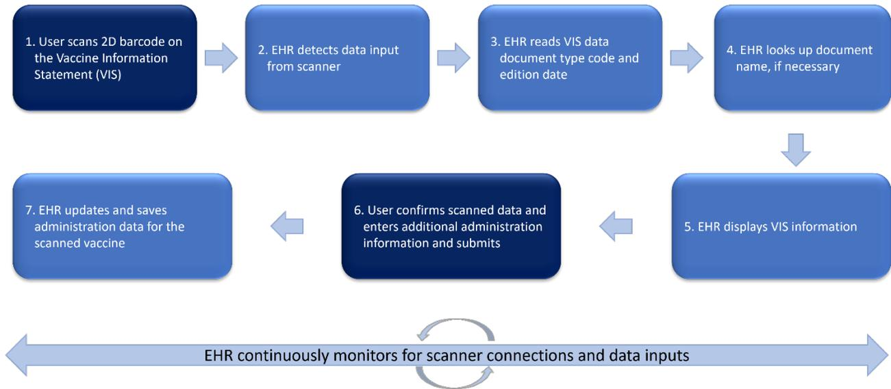
Figure 2: VIS Process Flow
