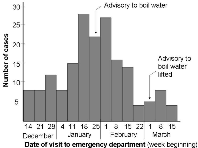
Changes at the water treatment facility improved the turbidity of treated water, consistently removing particles larger than approximately 1 micrometer. *Cryptosporidium* oocysts are approximately 3–4  $\mu\text{m}$  in size. A sample of water taken on February 11 revealed no oocysts. The consistently low turbidity readings resulted in the lifting of the boil-water advisory on March 2.
