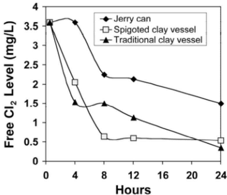
FIGURE 2— Free chlorine (Cl<sub>2</sub>) levels in river water treated with 16 mL (8 mg/L) of 1% sodium hypochlorite solution, by time interval: Laboratory study, Ariri, Kenya, May 2000.
