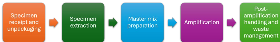
Figure A1. Hypothetical PCR workflow illustrating key stages from specimen receipt through post-amplification handling and waste management.
