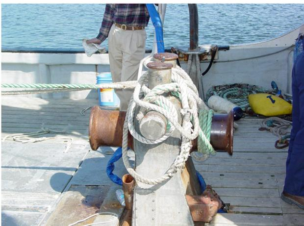
Fig. 2. Photo of capstan-type winch with lines around, F/V Lake Bay.
