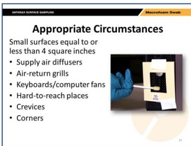
If you need to sample an area that is not square, use tape to outline an area that does not exceed 4 square inches. You can sample an area less than 4 square inches, but you should not sample an area that is larger. Be sure to make a note on the sampling sheet when you use an area other than 4 square inches; this information is needed to help analyze the sample and interpret the results.
