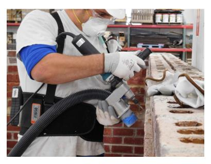
Figure 2 – Die grinder with on-tool exhaust hood (NIOSH photo)
