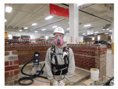
Figure 5 - Worker wearing air samplers
