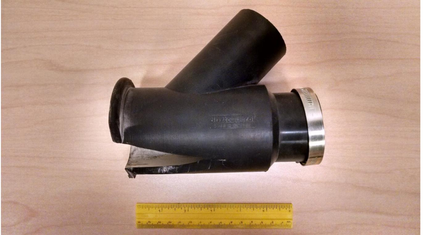
**Figure 3 - On tool exhaust hood (NIOSH photo)**
