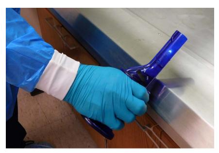
Figure 8. Example of a qualitative smoke test with Wizard Stick Smoke Generator (Photo Credit: NIOSH)
