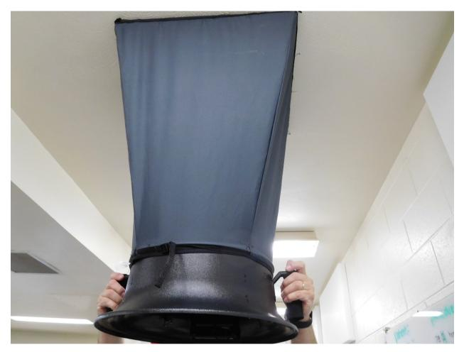
Figure 11. TSI Accubalance<sup>®</sup> Plus Air Capture Hood (Photo Credit: NIOSH)
