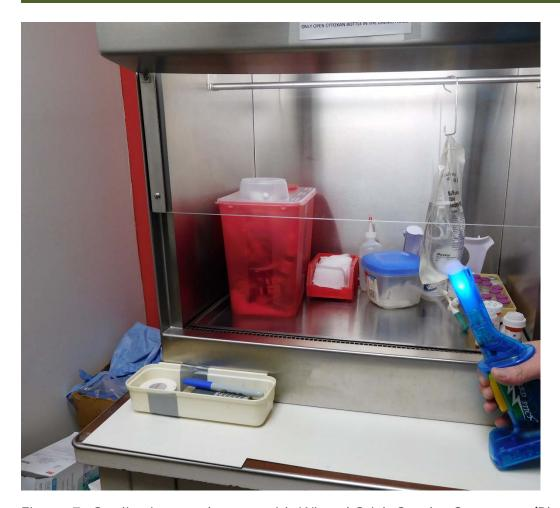
Figure 7. Qualitative smoke test with Wizard Stick Smoke Generator (Photo Credit: NIOSH)
