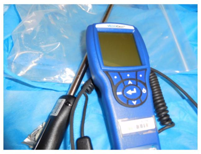
Figure 6.  $TSI^{\otimes}$  VelociCalc $^{\text{\tiny{M}}}$  Plus Model 9555-P thermal anemometer (Photo Credit: NIOSH)
