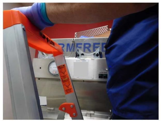
Figure 21. Wipe sample collected on HEPA filter box surface (Photo credit: NIOSH)
