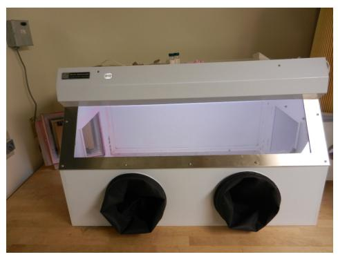
Figure 5. Glovebox used for lab testing, showing access door open at left.
