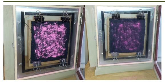
Figure 15. An example of the appearance of the test swatch before and after one of the most successful decontamination trials, using the leaf blower without hose.
