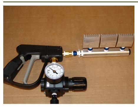
Figure 9. Norgren pressure regulator and Spraying Systems spray gun attached to a manifold with 3 Air TX spray nozzles (configuration 1).
