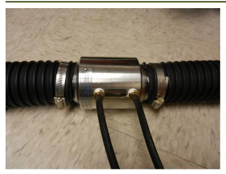
Figure 7. Primary Flow Signal flowmeter, used to measure the flow rate of low-pressure air.
