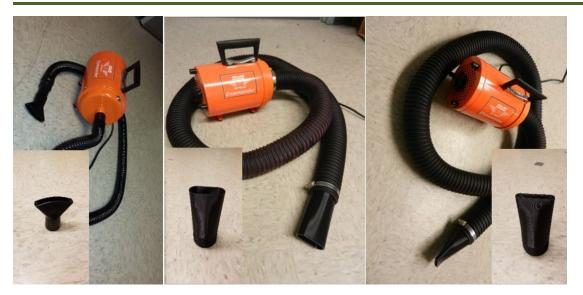
Figure 13. Three different configurations of the Metro pet dryer were tested: as sold with a narrow hose and fan-shaped nozzle, with a larger hose and a wide -slot nozzle, and with the larger hose and a narrow-slot nozzle.
