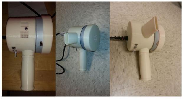
Figure 12. Three different housings tested with high-speed hand dryer blower: outlet holes, wide-slot nozzle and narrow-slot nozzle.
