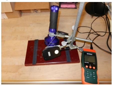
Figure 1. The blacklight flashlight and light meter sensor used in testing were attached to a ring stand to obtain reproducible readings of light intensity.
