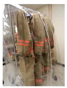
Figure 22. Fire-worn turnout gear inside an enclosure during collection of air samples for offgassing analysis.
