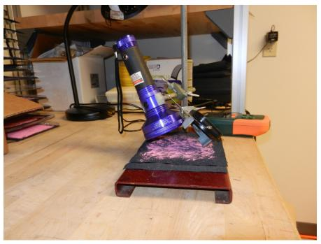
Figure 2. Fabric strips attached to the base of the ring stand allowed fabric squares to be positioned in the same location for each reading.
