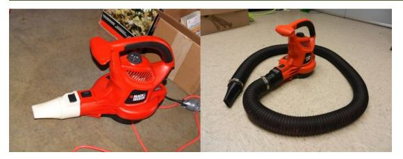
Figure 11. Modified leaf blower used for dry decontamination, with and without hose.
