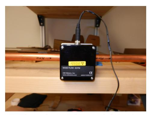
Figure 6. CDI mass flowmeter used to measure the flow rate of compressed air.
