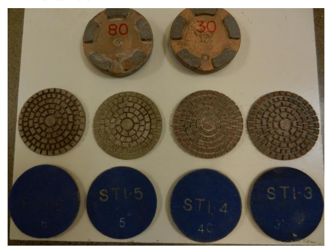
Figure 4: Different Grits used during the survey
