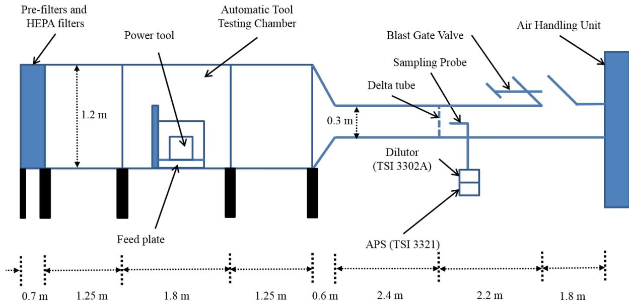
**Figure 1. Diagram of the Laboratory Testing System.**
