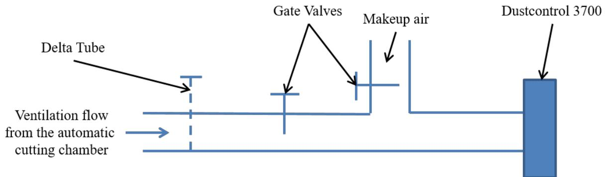
Figure 2. Diagram of the Local Exhaust Ventilation (LEV) system used in this study.
