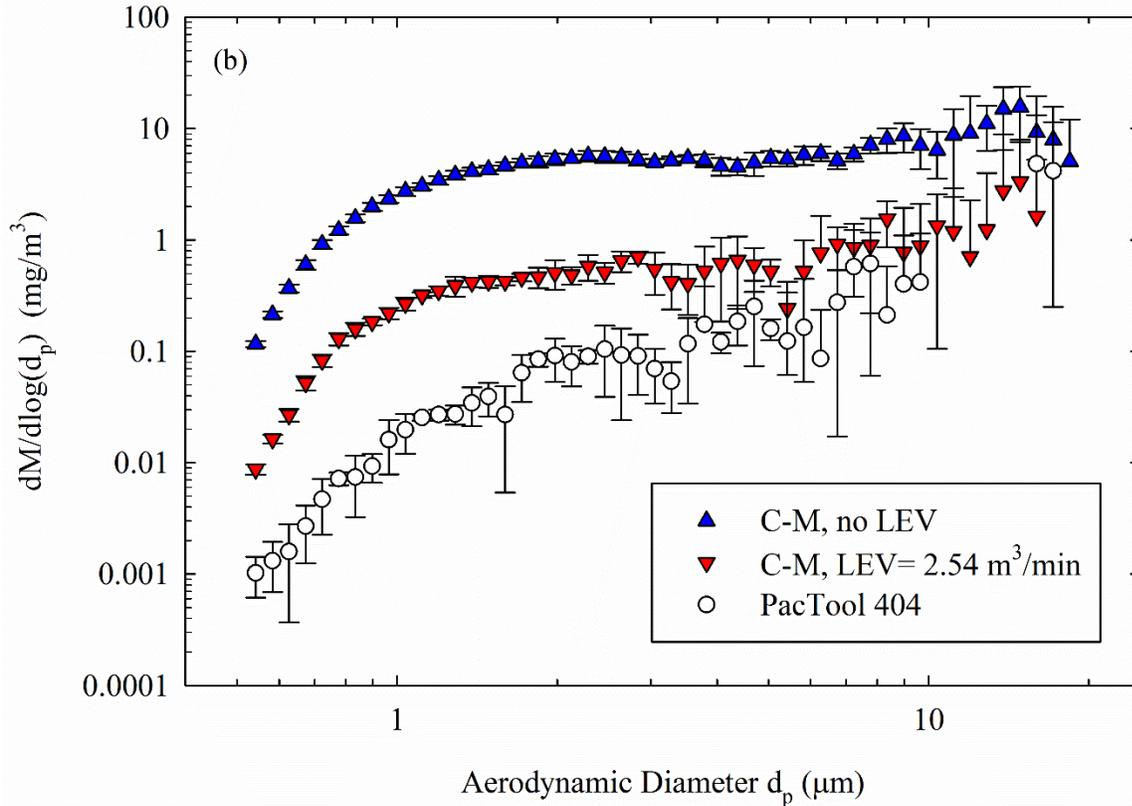
**Figure 3. Size distributions of the dust from cutting fiber-cement siding obtained from the APS (a) number-based; (b) mass-based. Cutting feed rate: 2.54 cm/sec.**
