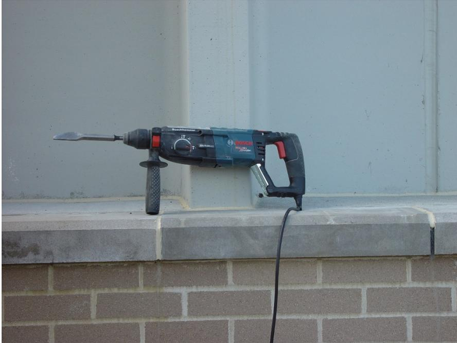
Figure 2 - Chisel Tool and Rotary Hammer (NIOSH photo)
