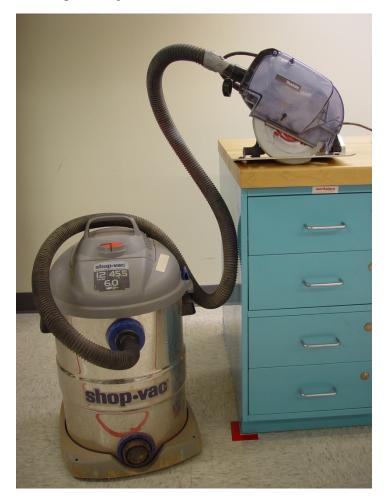
Figure 3 – The dust-collecting circular saw and its connection to the shop vacuum used in this survey. Photo courtesy of NIOSH.
