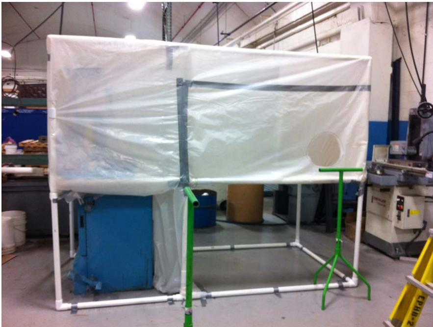
Figure 4. Side view of enclosure around band saw. The hole in the enclosure above the support stand is where the elbow was inserted into the enclosure.
