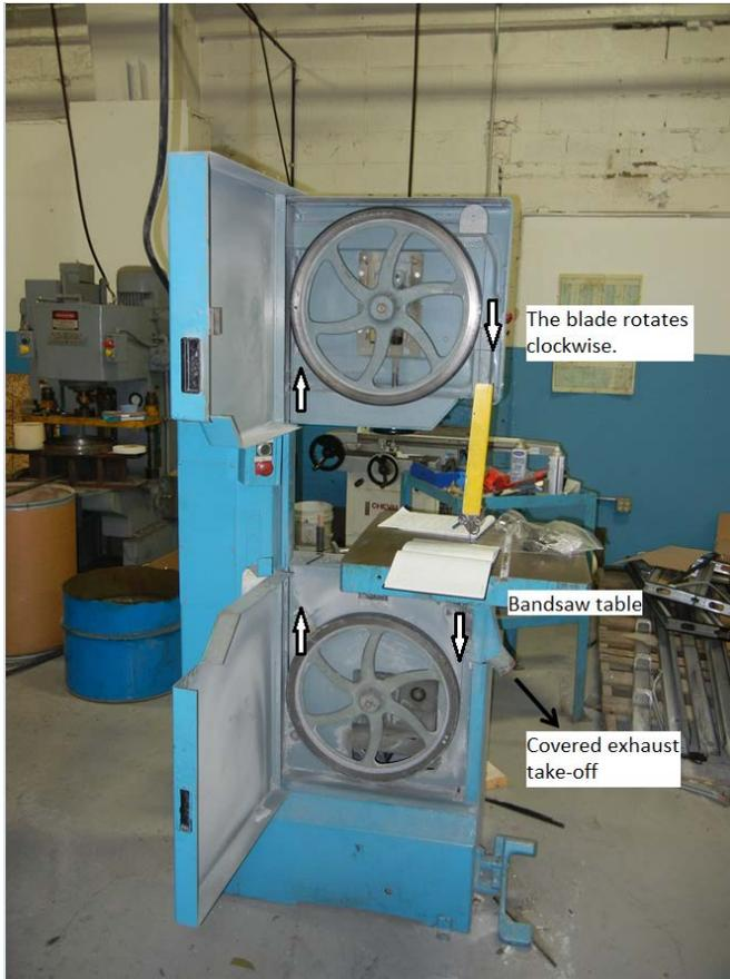
Figure 1. Bandsaw with access doors open.
