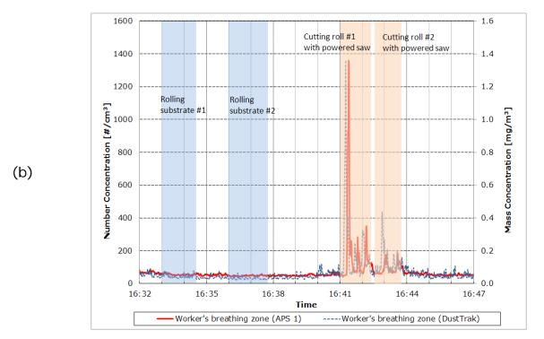
Figure 12. Process monitoring by (a) FMPSs, and (b) APS 1 and DustTrak, for rolling substrates on the downdraft table and cutting rolls by the powered circular saw with the canopy hood off (normal operation) on 04/27.
