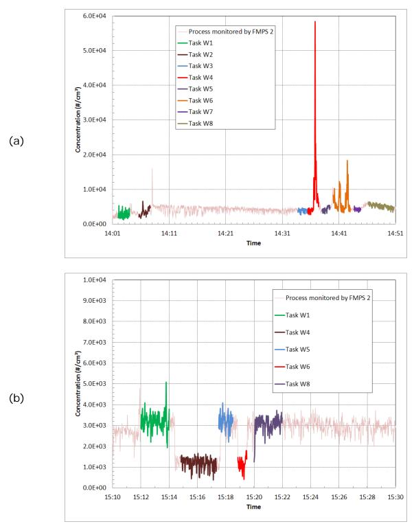
Figure 8. Evaluation of the laboratory hood for the CNT weighing process, when the hood fan was turned (a) off, and (b) on.
