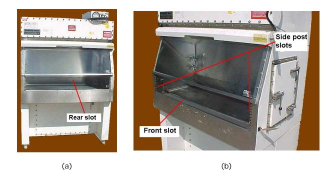
**Figure 3**: (a) Front view and (b) side view of Baker BioGARD Class II type B2 lab environmental hood. A similar lab hood was used at the study site for weighing CNTs. (photos taken from http://www.bid-on-equipment.com/detail~id~102174.htm#).
