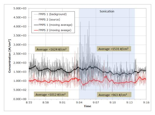
Figure 16. Sonication chamber monitored with FMPSs on 04/28.
