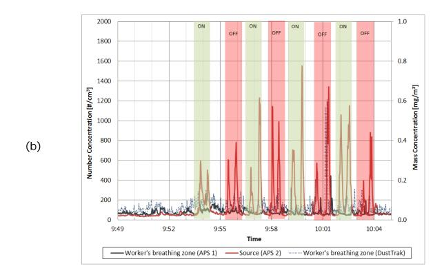
Figure 14. Particle concentration monitoring data of (a) FMPSs, and (b) APSs and DustTrak during the evaluation of the canopy hood used for the powered saw cutting.
