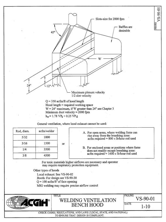
Figure 18. Ventilated bench hood design to control emissions from manual cutting of substrate materials using the rotary cutter [ACGIH 2010].
