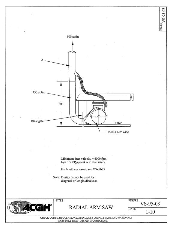
Figure 19. LEV designs to control dust emissions from the powered radial saw [ACGIH 2010].
