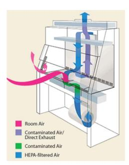
**Figure 4**. Airflow pattern for a Type II Biological Safety Cabinet. (Figure taken from http://www.bakerco.com/intro-to-biological-safety-cabinets.html)
