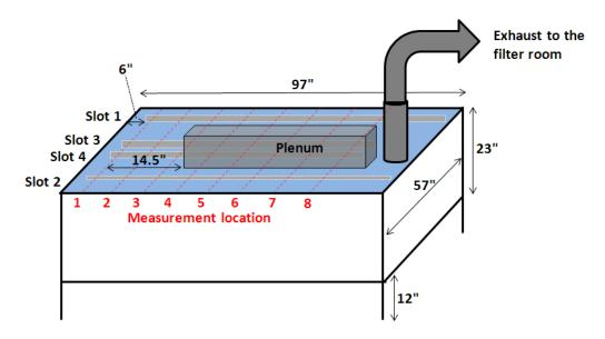
Figure 5: Top view of the downdraft table.
