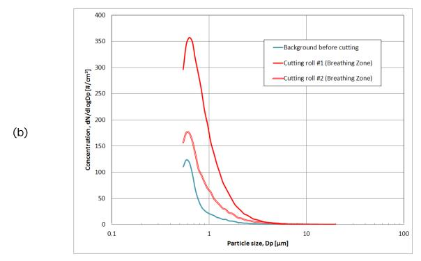
Figure 13. Particle size distribution analysis from (a) FMPSs and (b) APS 1 during the cutting of substrate rolls using the powered circular saw.
