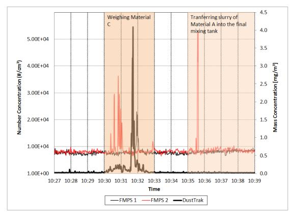
**Figure 9**: Monitoring the mixing process with FMPSs and DustTrak on 04/27.
