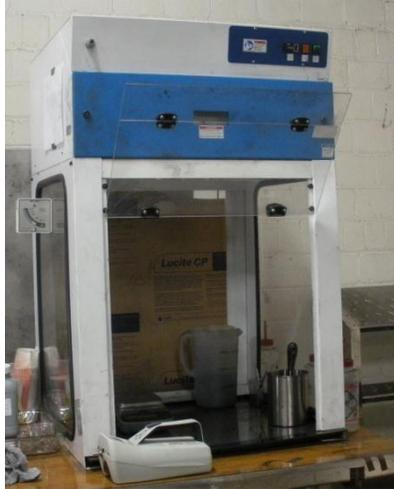
**Figure 3:** Ventilated enclosure used to weigh and transfer products in refining area.
