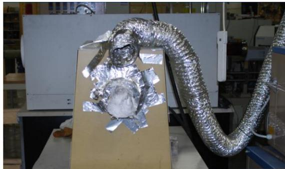
**Figure 4:** Local exhaust ventilation used in the post-treatment area.
