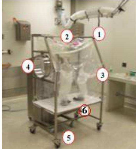
**Figure 25:** Flexible enclosure. Main components are marked by numbers: (1) enclosure, (2) HEPA filters, (3) integral glove sleeves, (4) entry/removal door, (5) conductive locking castors, and (6) support table. (Reprint from [ILC Dover, 2009])
