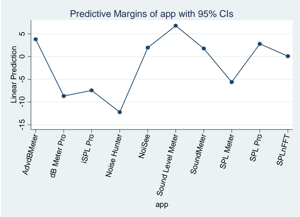
Figure 6. Marginal predicted means of differences in unweighted sound levels (dB) for the ten apps.
