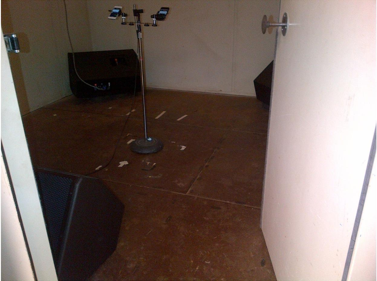
**Figure 1. View of the setup inside the reverberant chamber showing the speakers and the smartphones stand with the reference microphone.**
