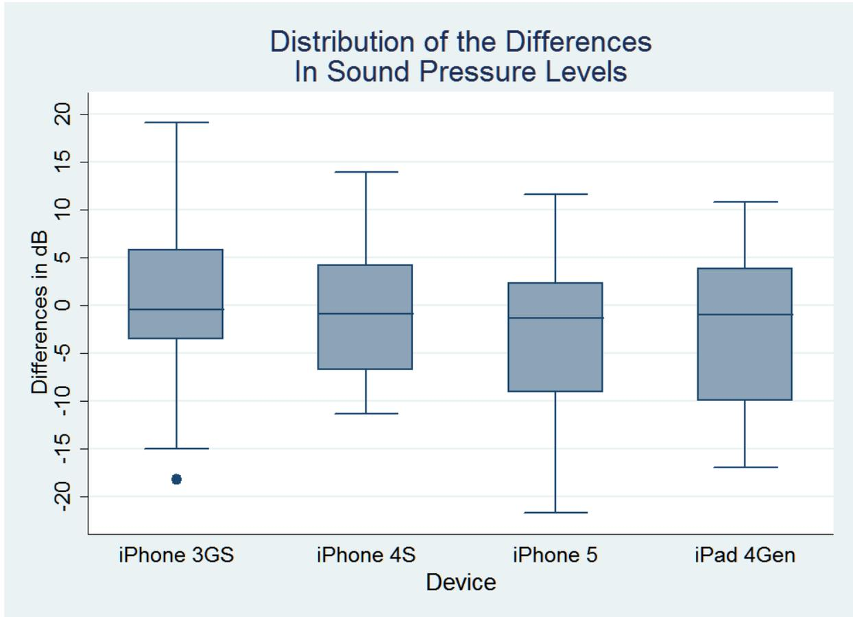
**Figure 8. Box plots of differences in unweighted sound levels (dB) between reference microphone and app measurements by device.**
