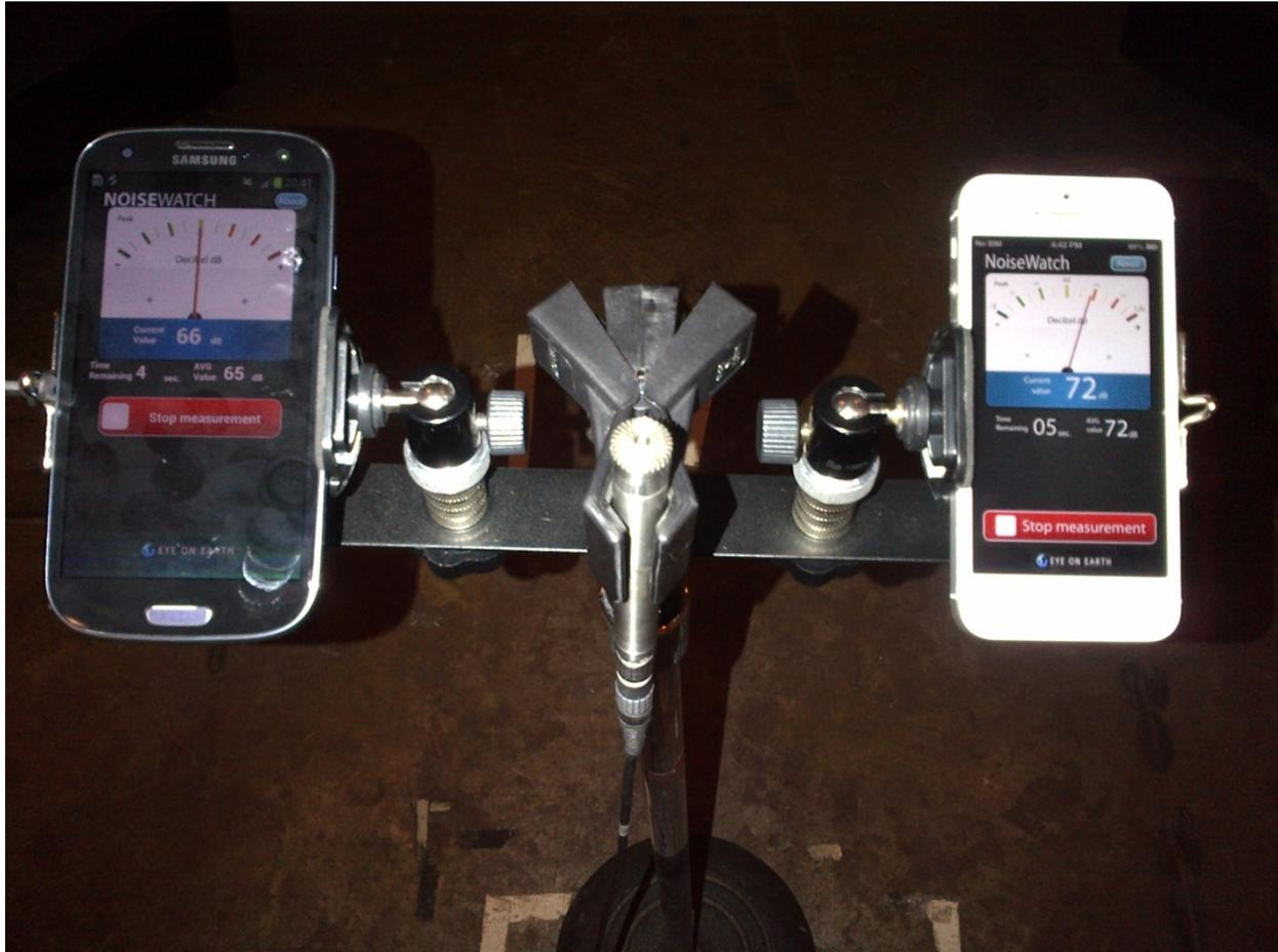
Figure 9. NoiseWatch app on the Samsung S3 Android device (left) and the iPhone 5 (right).
