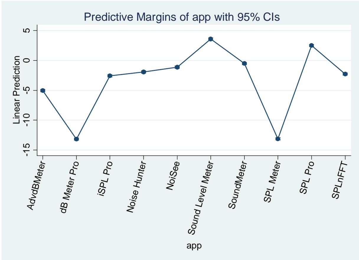
Figure 3. Marginal predicted means of differences in dBA for the ten apps.
