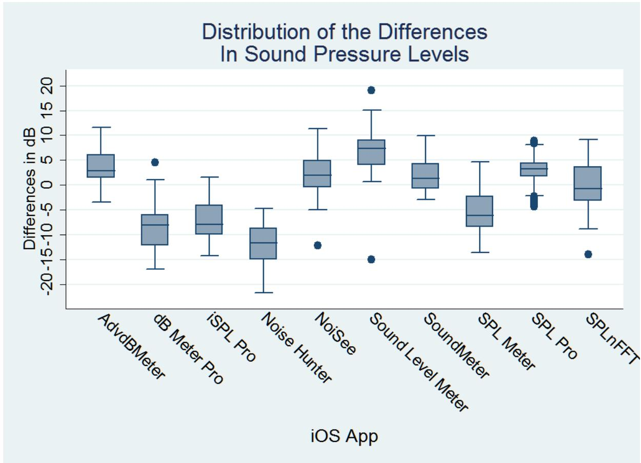
Figure 7. Box plots of differences in unweighted sound levels (dB) between reference microphone and app measurements by app.
