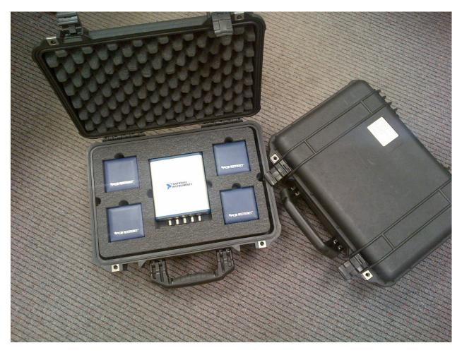
Figure 1. NIOSH Impulsive Noise Measurement Kit
