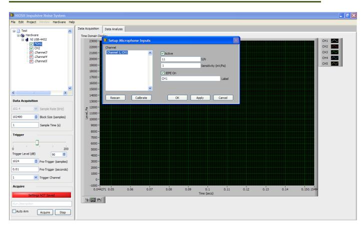
Figure 5. Individual Channel Setup
