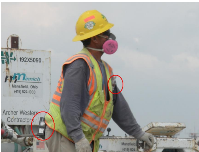
Figure 2 - Worker Wearing Pump and Cyclone (Circled)
