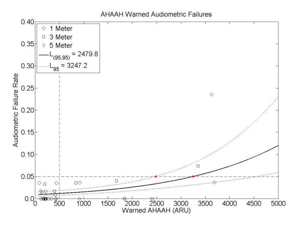
Figure 10: Evaluations of 1, 3 and 5-meter exposures using the warned AHAAH model using the audiometric failures. The logistic regression curve and 95% confidence intervals are shown as the solid and dotted lines. The  $L_{(95,95)}$  and  $L_{95}$  points are plotted with a solid dot symbol. The 5% failure criterion and the 500 ARU suggested damage-risk criterion are shown as horizontal and vertical dashed-dotted lines.
