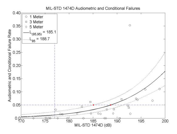
Figure 3: Evaluations of 1, 3 and 5-meter exposures using the MIL-STD-1474D metric using the audiometric and conditional failures. The logistic regression curve and 95% confidence intervals are shown as the solid and dotted lines. The  $L_{(95,95)}$  and  $L_{95}$  points are plotted with a solid dot symbol. The 5% failure criterion and the 177 dB design limit are shown as horizontal and vertical dashed-dotted lines.
