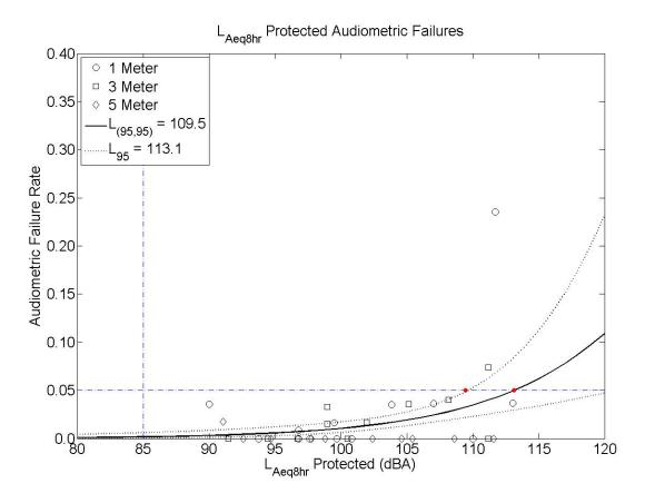
Figure 6: Evaluations of 1, 3 and 5-meter exposures using the protected 8-hour equivalent Aweighted Level,  $L_{Aeq8hr}$ , metric using the audiometric failures. The logistic regression curve and 95% confidence intervals are shown as the solid and dotted lines. The  $L_{(95,95)}$  and  $L_{95}$ points are plotted with a solid dot symbol. The 5% failure criterion and the 85 dBA suggested damage-risk criterion are shown as horizontal and vertical dashed-dotted lines.
