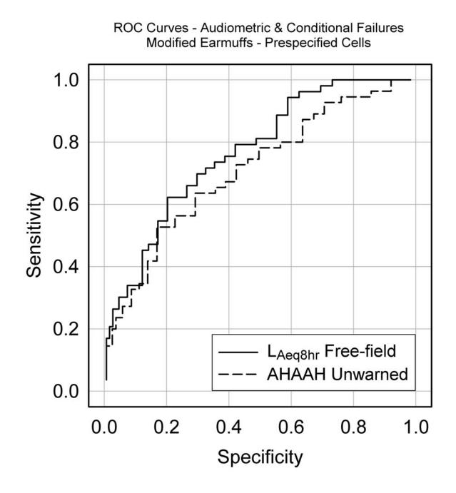
Figure 13: ROC curves for audiometric and conditional failures combined for pre-specified cells for  $L_{Aeq8hr}$  and unwarned AHAAH damage-risk criteria.
