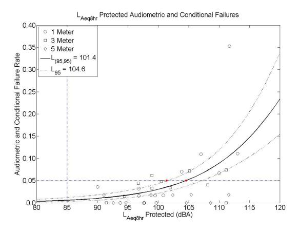
Figure 7: Evaluations of 1, 3 and 5-meter exposures using the protected 8-hour equivalent Aweighted Level,  $L_{Aeq8hr}$ , metric using the audiometric and conditional failures. The logistic regression curve and 95% confidence intervals are shown as the solid and dotted lines. The  $L_{(95,95)}$  and  $L_{95}$  points are plotted with a solid dot symbol. The 5% failure criterion and the 85 dBA suggested damage-risk criterion are shown as horizontal and vertical dashed-dotted lines.
