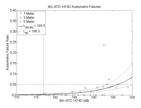
Figure 2: Evaluations of 1, 3 and 5-meter exposures using the MIL-STD-1474D metric using the audiometric and conditional failures. The logistic regression curve and 95% confidence intervals are shown as the solid and dotted lines. The  $L_{(95,95)}$  and  $L_{95}$  points are plotted with a solid dot symbol. The 5% failure criterion and the 177 dB design limit are shown as horizontal and vertical dashed-dotted lines.
