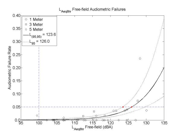
Figure 4: Evaluations of 1, 3 and 5-meter exposures using the protected 8-hour equivalent Aweighted Level,  $L_{Aeq8hr}$ , metric using the audiometric failures. The logistic regression curve and 95% confidence intervals are shown as the solid and dotted lines. The  $L_{(95,95)}$  and  $L_{95}$ points are plotted with a solid dot symbol. The 5% failure criterion and the 100 dBA limit (85 dBA protected DRC+ 15 dBA hearing protection) are shown as horizontal and vertical dasheddotted lines.
