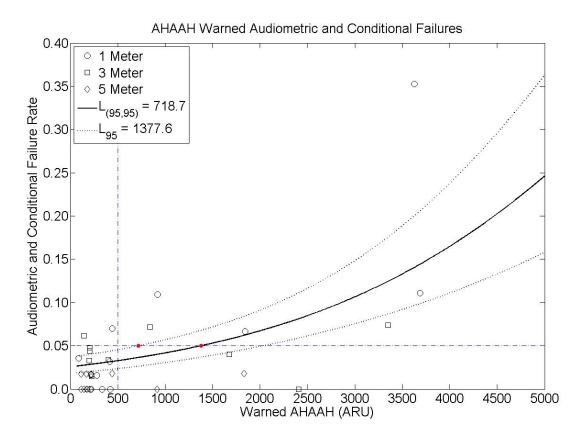
Figure 11: Evaluations of 1, 3 and 5-meter exposures using the warned AHAAH model using the audiometric and conditional failures. The logistic regression curve and 95% confidence intervals are shown as the solid and dotted lines. The  $L_{(95,95)}$  and  $L_{95}$  points are plotted with a solid dot symbol. The 5% failure criterion and the 500 ARU suggested damage-risk criterion are shown as horizontal and vertical dashed-dotted lines.
