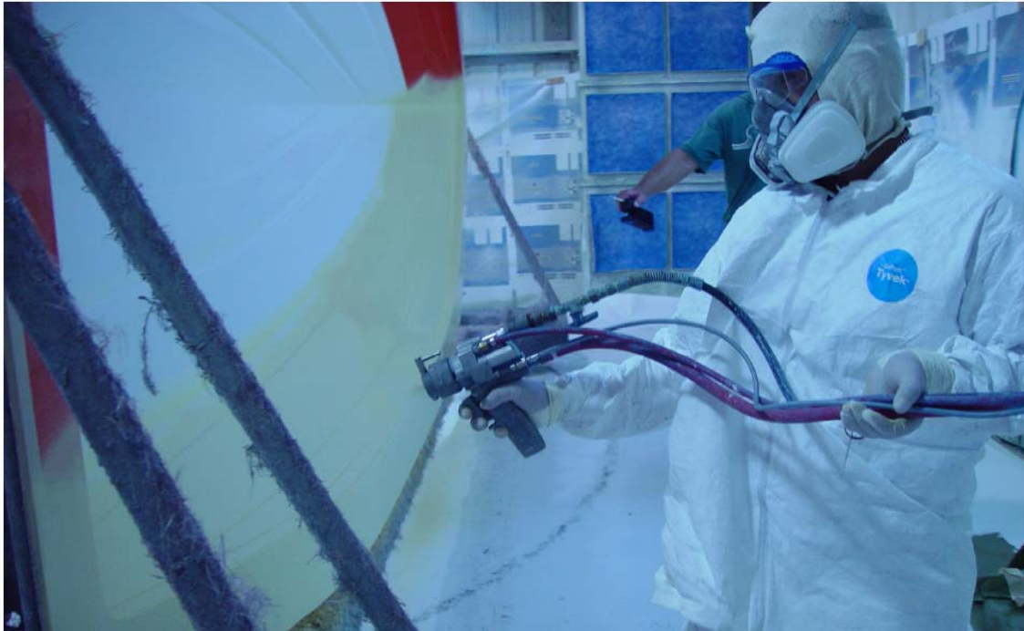
Figure 3: Gelcoater spraying a production hull
