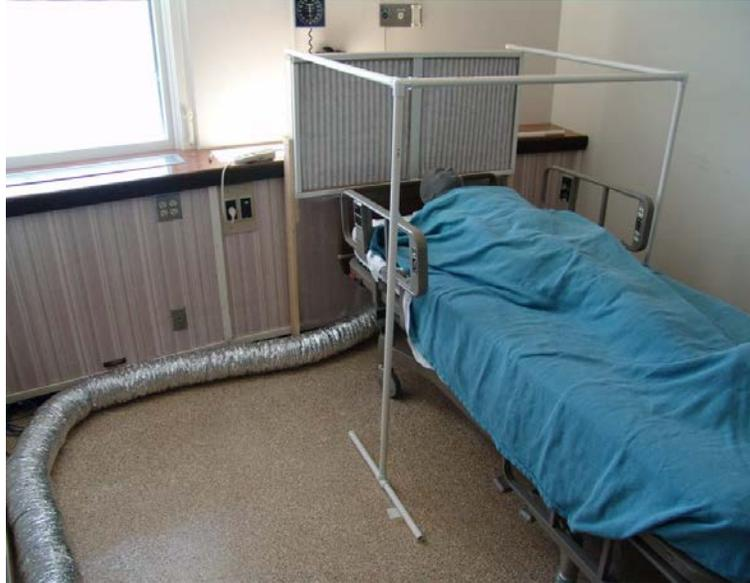
Figure 25. Photograph of ventilated headboard and hood frame as constructed for research at the Central Kansas Medical Center, in Great Bend, KS.
