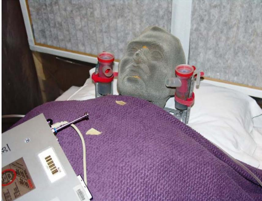
Figure 6. Photo of patient mannequin positioned in front of a ventilated headboard shows source generators (nebulizers) positioned next to the mannequin's mouth and an aerosol sampler positioned in the center of the mannequin's chest.
