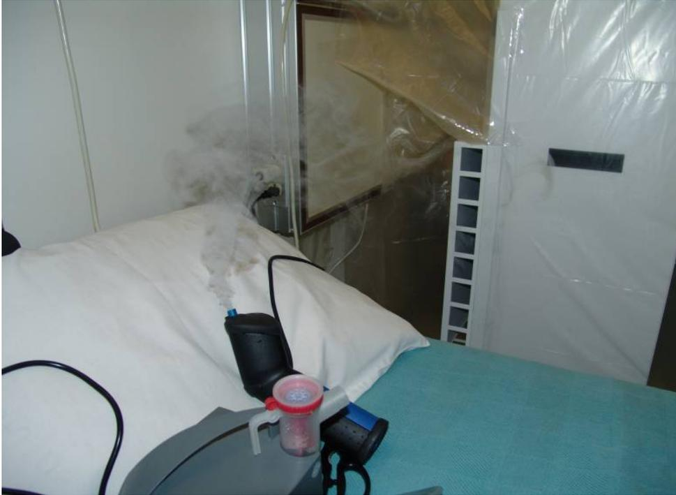
Figure 30. A photograph showing the HEPA filter unit's inlet position relative to that of the source patient's pillow position during a qualitative smoke capture test.
