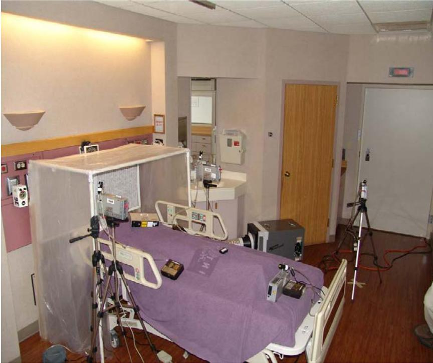
Figure 14. Photograph of ventilated headboard configuration as constructed for field research at the INTEGRIS Baptist Medical Center, in Oklahoma City, OK.
