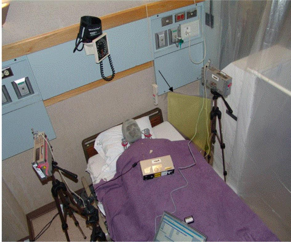
Figure 35. The HEPA filter unit's inlet position (and turbulence-reducing baffle) relative to the source patient's pillow position and aerosol spectrometer sampling positions A, C, and B.
