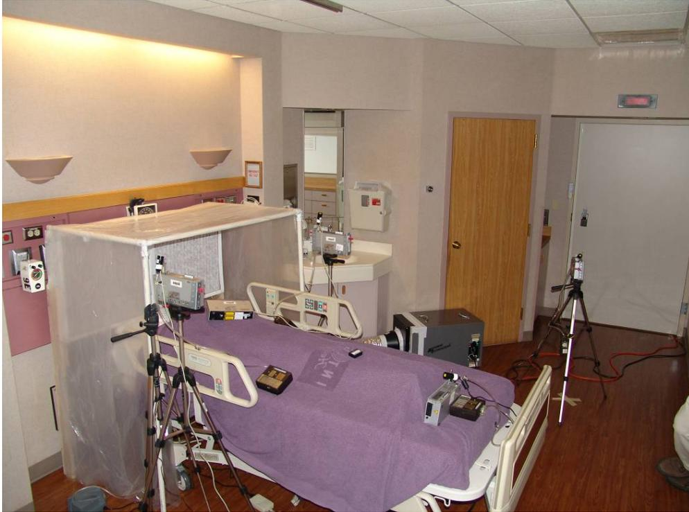
Figure 38. The ventilated headboard configuration as constructed for field research at the INTEGRIS Baptist Medical Center, in Oklahoma City, OK.
