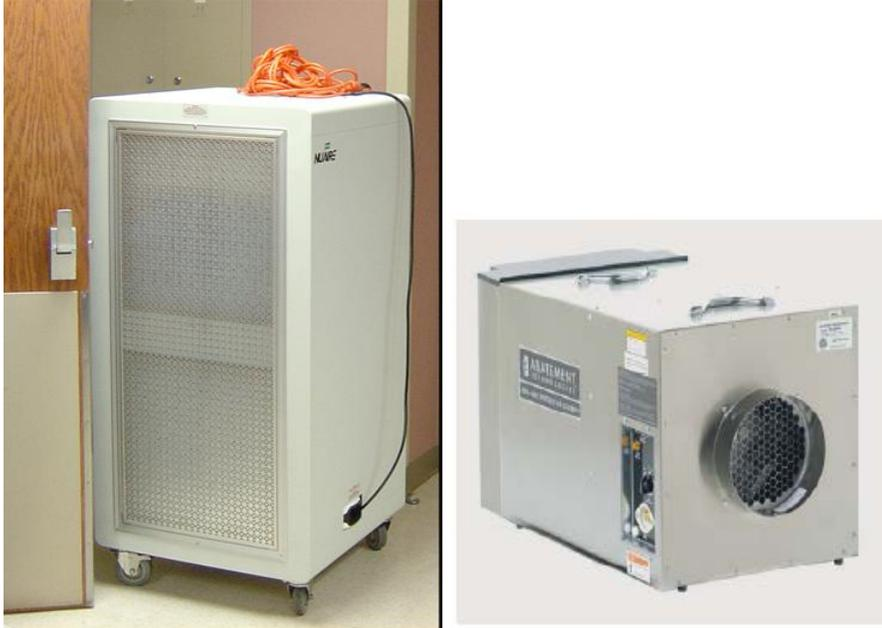
Figure 5. Photographs of some of the portable HEPA filtration equipment used during the expedient isolation research. A portable freestanding unit with nonducted inlet (*left*) and a portable dust-control unit, capable of ducted or freestanding operation (*right*).
