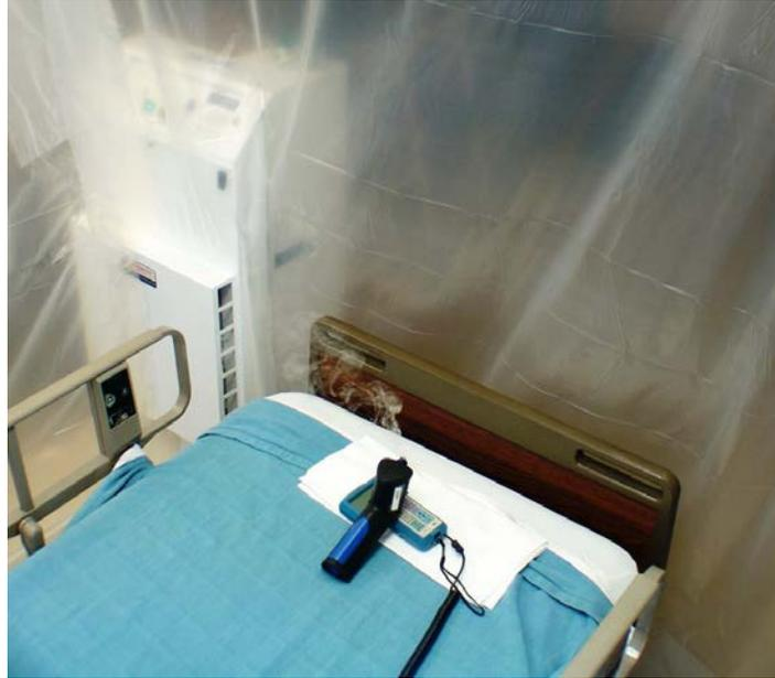
Figure 22. A photograph showing the HEPA filter unit's inlet relative to the source bed pillow position, during a qualitative smoke test at Central Kansas Medical Center, Great Bend.
