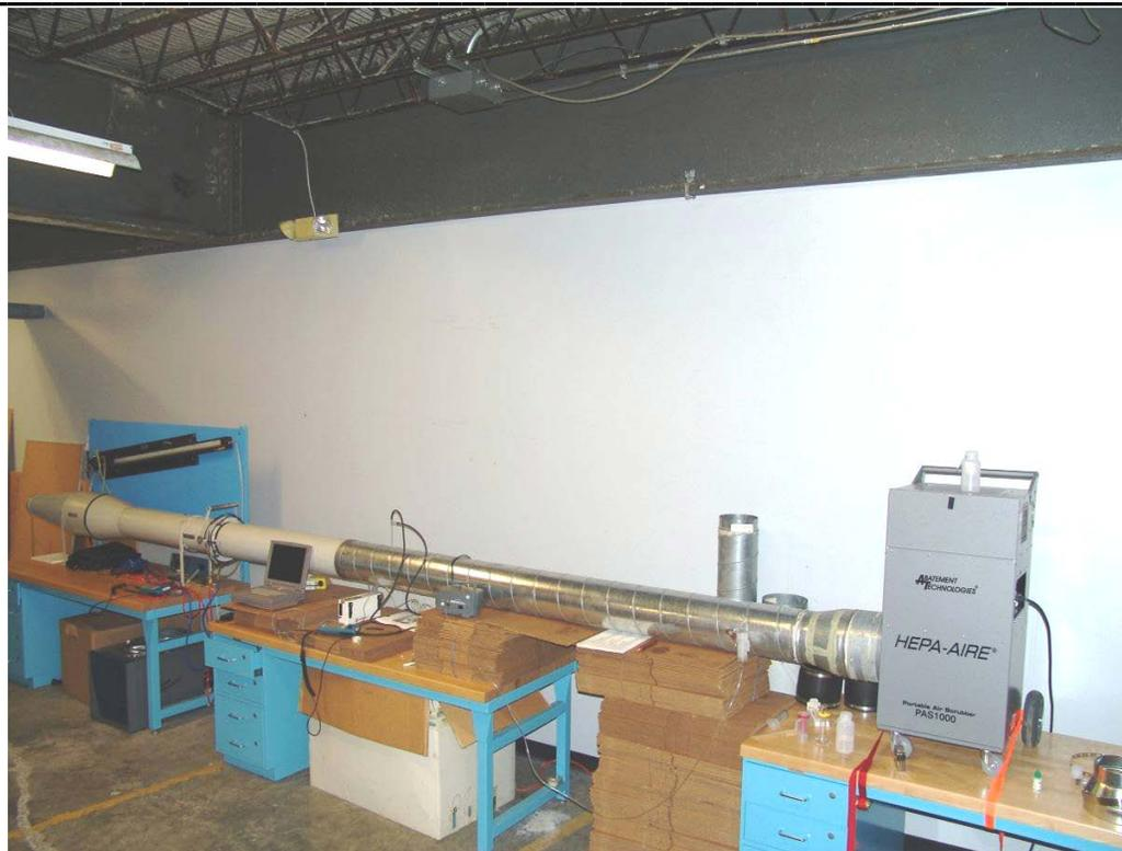
Figure 7. Schematic (7a) and photograph (7b) showing the testing platform used for development of the aerosol generation protocol.
