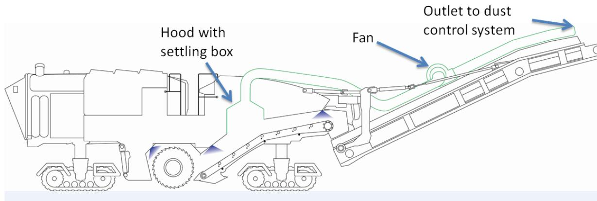
**Figure 1: Hood with settling box on a milling machine**
