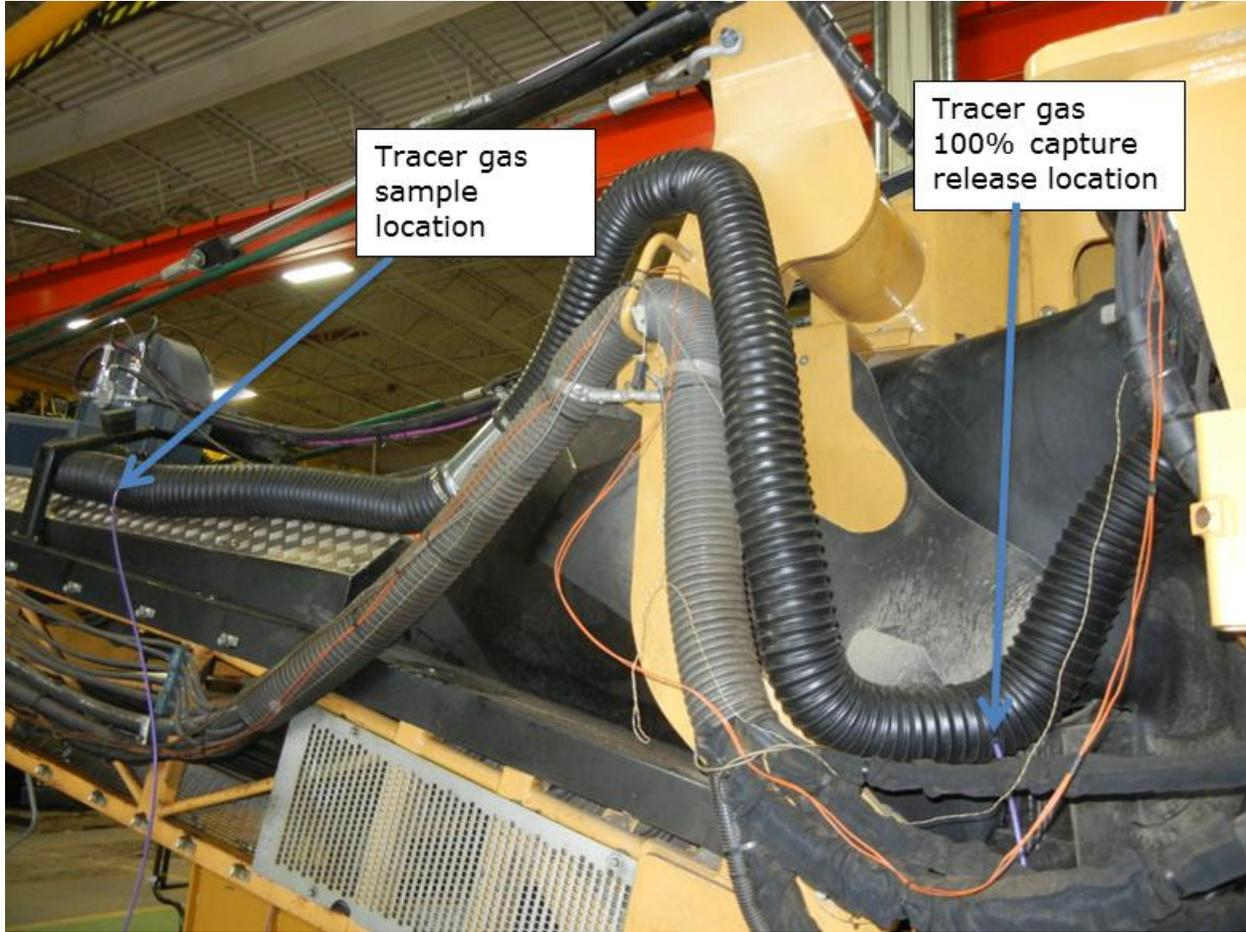
Figure 2: Tracer gas sampling and 100% release locations
