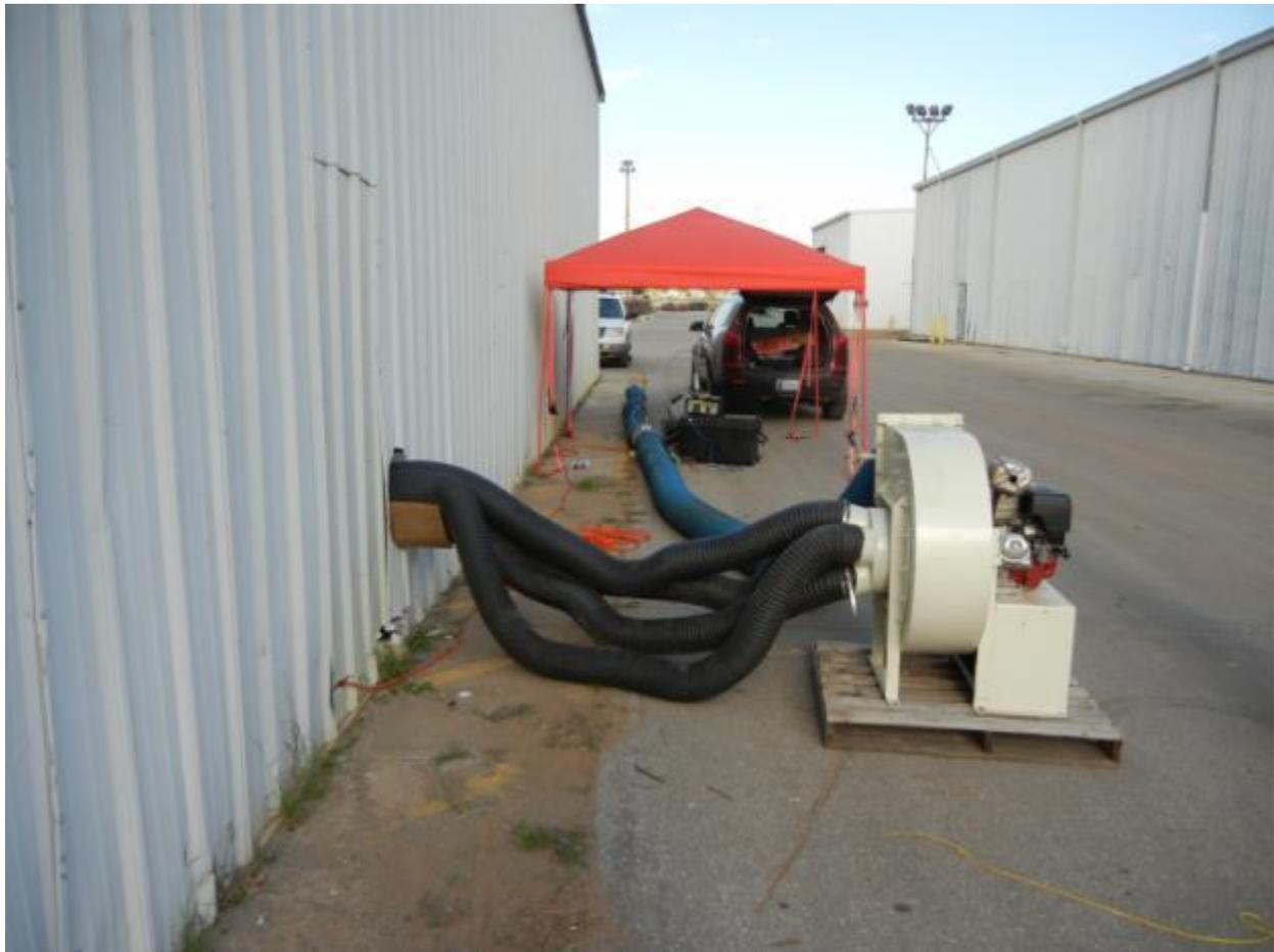
**Figure 2: Fan and ductwork for prototype LEV testing.**
