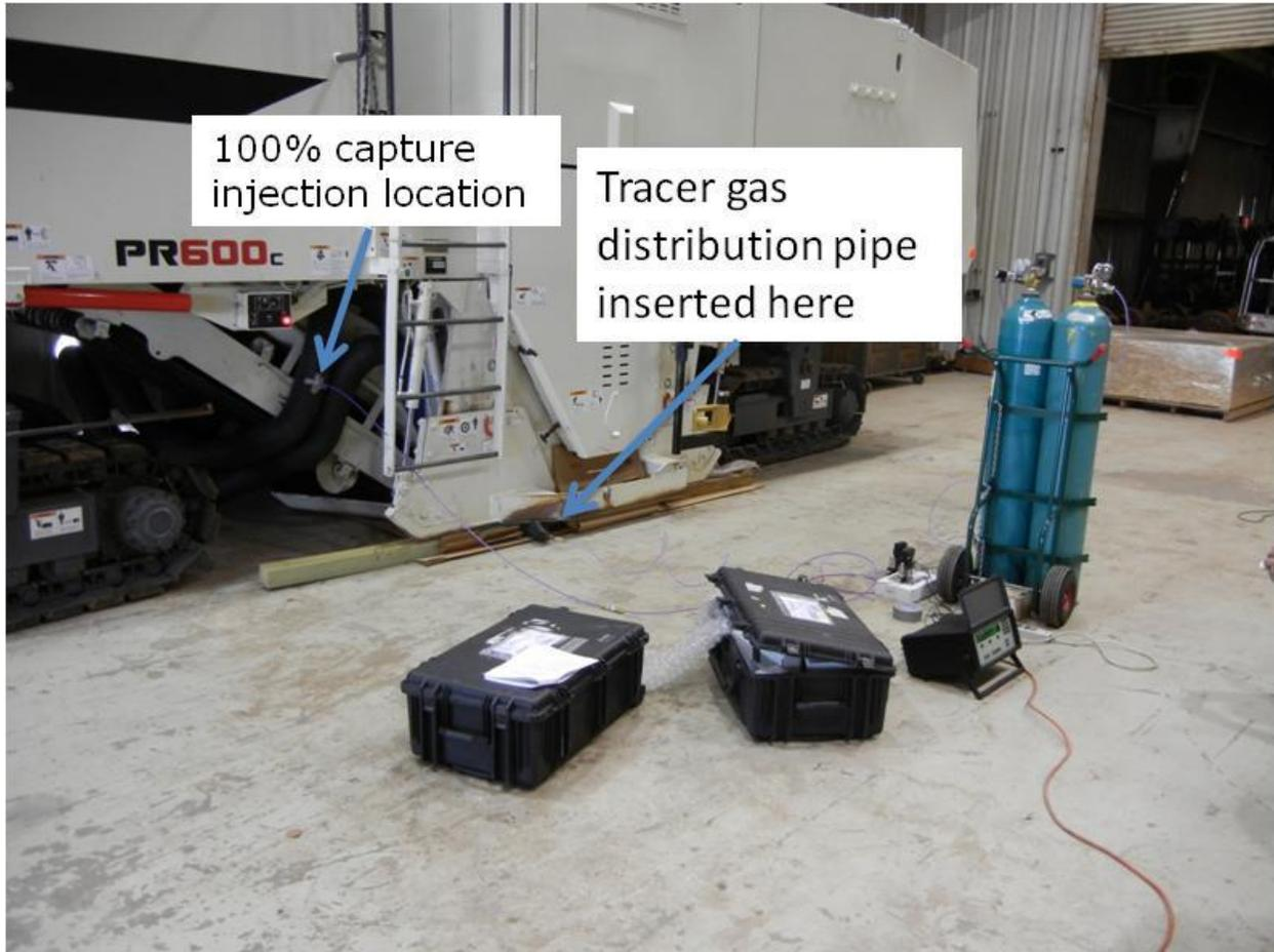
**Figure 3: Tracer gas injection locations.**
