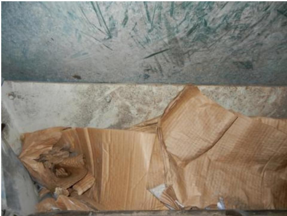
Figure 7: Obstruction stuffed in the outlet of the primary conveyor.
