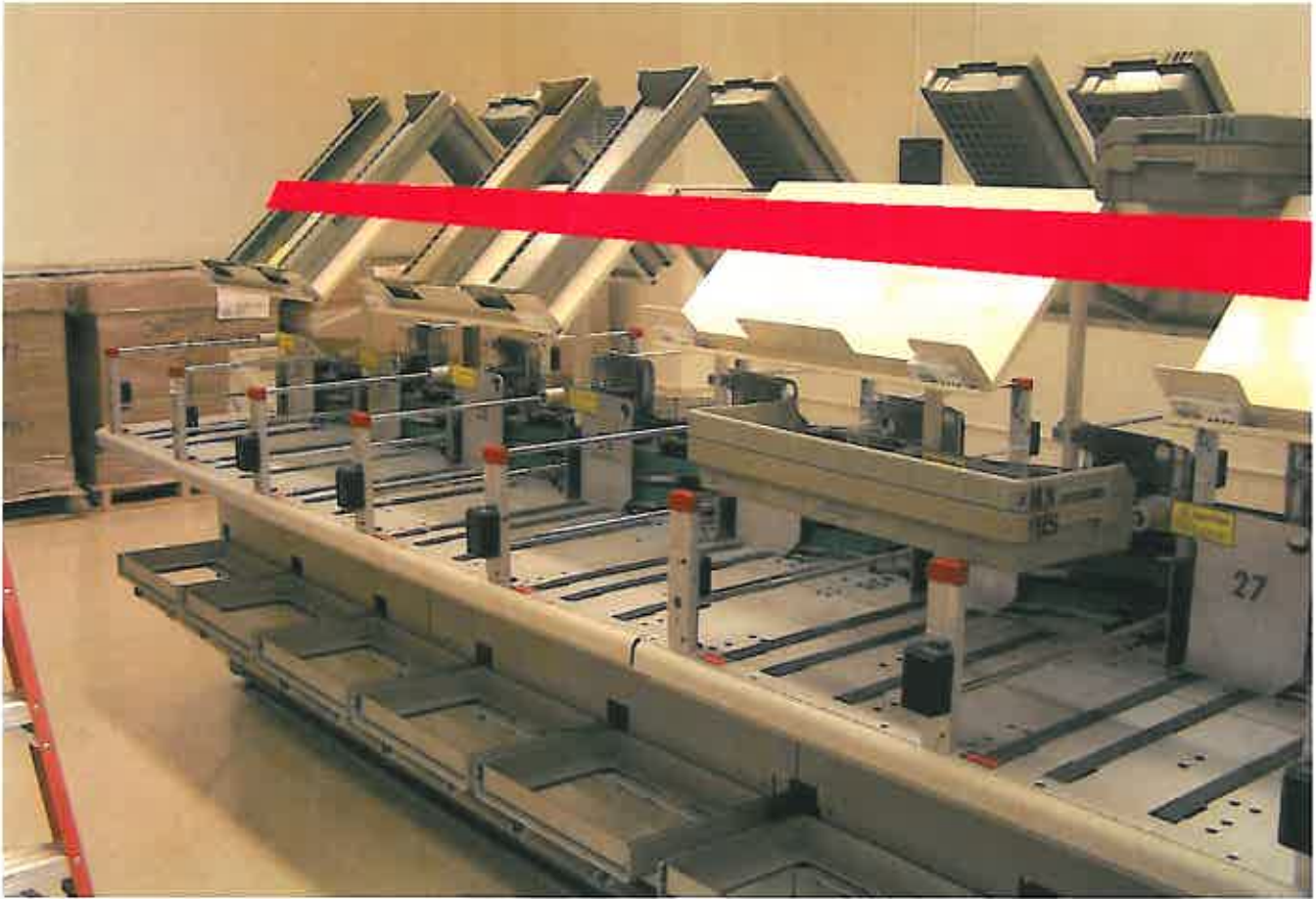
Figure 12. Schematic of Possible Location for LEV on SCAMPS Rooms Mail-Processing Machinery (the red strip signifies where LEV ductwork could be used to help entrain air away from the worker's breathing zone)
