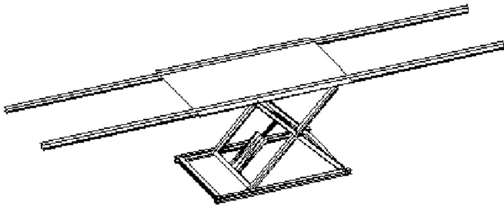
Figure 16. Lift Table with Jig Support Beams
