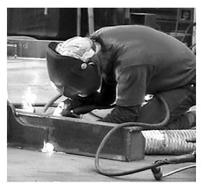
Figure 14. Panel Line Welder Wire Welding
