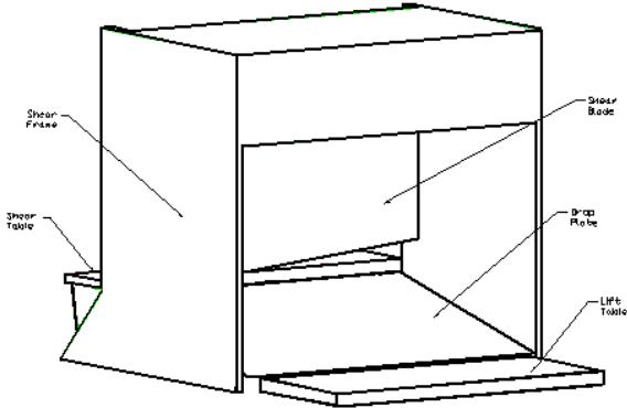
Figure 11: Shear with Lift Table in Down Position
