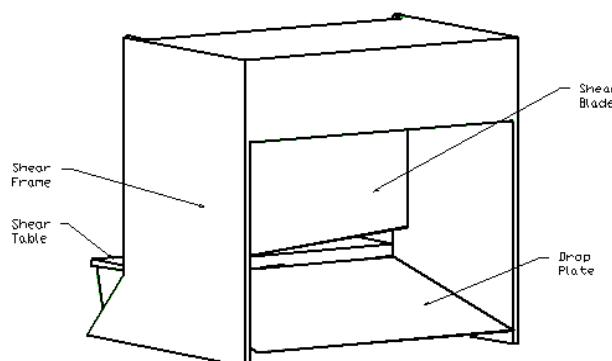
Figure 10: Oblique Rear View of Shear
