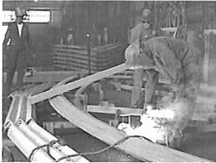
Figure 7. Welding rake frame angle irons while standing
