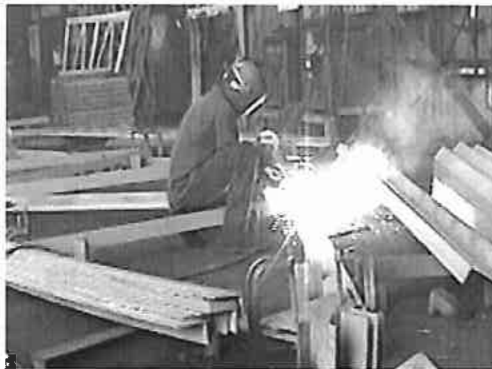
Figure 8. Welding rake frame angle irons while squatting
