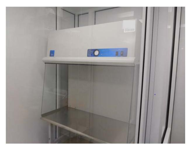
Figure 1. Labconco Laminar Air Flow Work Station (Photo Credit: NIOSH)
