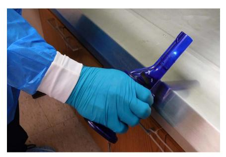
Figure 4. Example of a qualitative smoke test with Wizard Stick Smoke Generator (Photo Credit: NIOSH)
