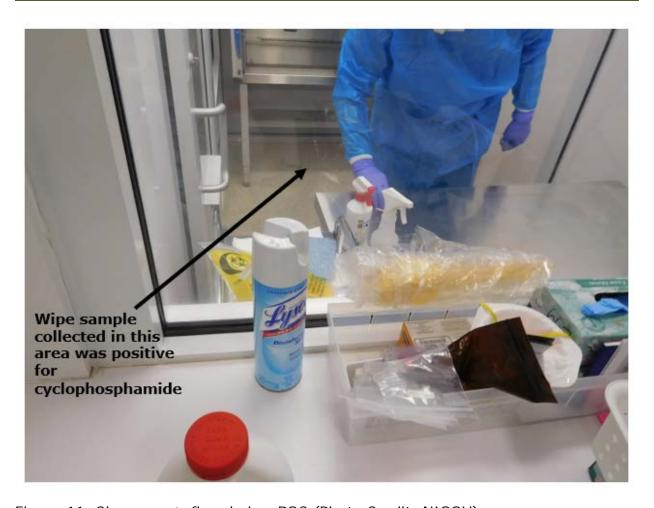
Figure 11. Cleanroom's floor below BSC (Photo Credit: NIOSH)
