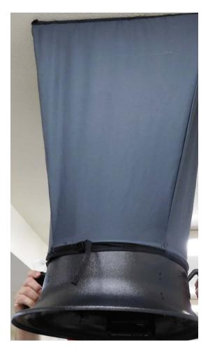
Figure 6. TSI Accubalance<sup>®</sup> Plus Air Capture Hood (Photo Credit: NIOSH)
