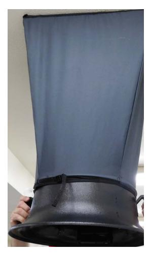
Figure 9. TSI Accubalance<sup>®</sup> Plus Air Capture Hood (Photo Credit: NIOSH)
