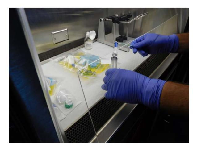
Figure 27. Intentional "Hot" wipe sample collected from carboplatin syringe with CSTD adapter. Also shown: PhaSeal vial adapter and adsorbent pad. (Photo Credit: NIOSH)
