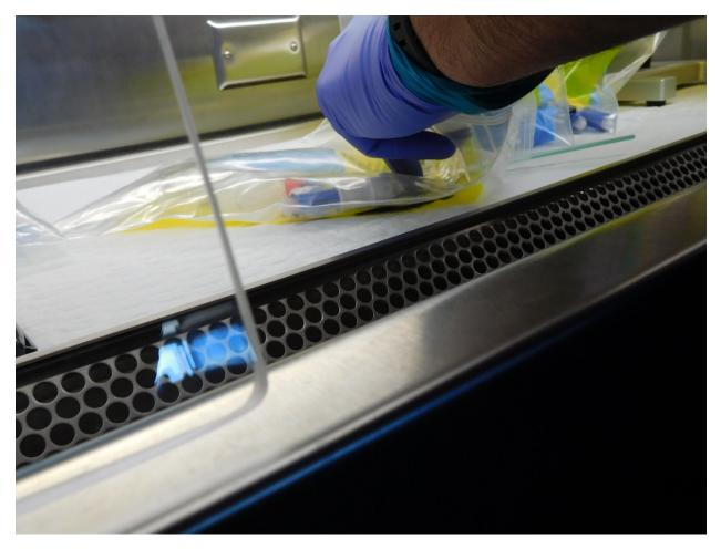
Figure 31. Sample collection from outside of chemo transport bag containing doxorubicin syringe with CSTD adapter. An intentional "Hot" wipe sample was also collected from the doxorubicin syringe. (Photo Credit: NIOSH)
