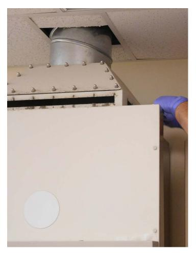
Figure 10. Surface wipe sample collected downstream of BSC's HEPA filter (Photo Credit: NIOSH)
