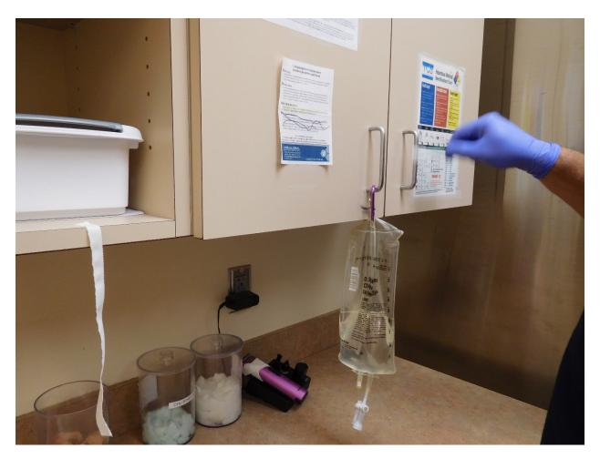
Figure 12. Surface wipe sample collected from storage cabinet handle (Photo Credit: NIOSH)
