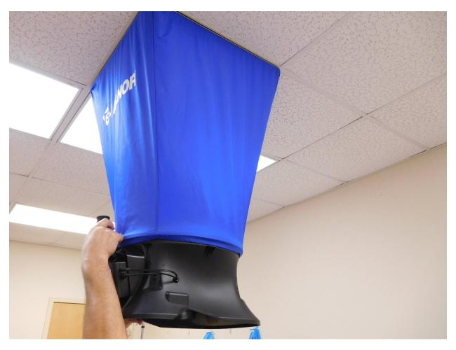
Figure 6. TSI Accubalance® Plus Air Capture Hood (Photo Credit: NIOSH)
