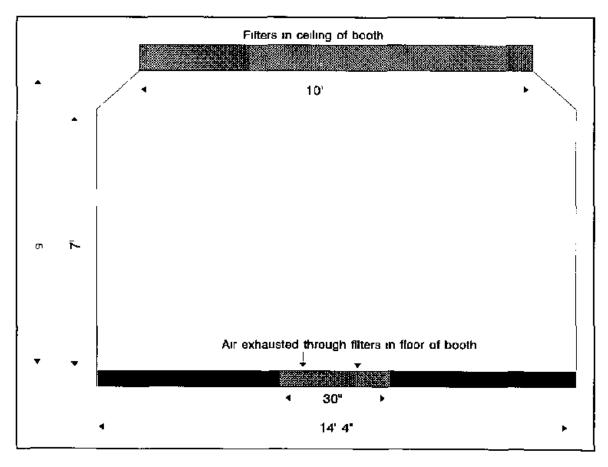
Figure 2 Cross sectional view of a spray painting booth during second set of tests - Instead of the normal two exhaust trenches, this booth has a single exhaust trench in the floor of the booth
