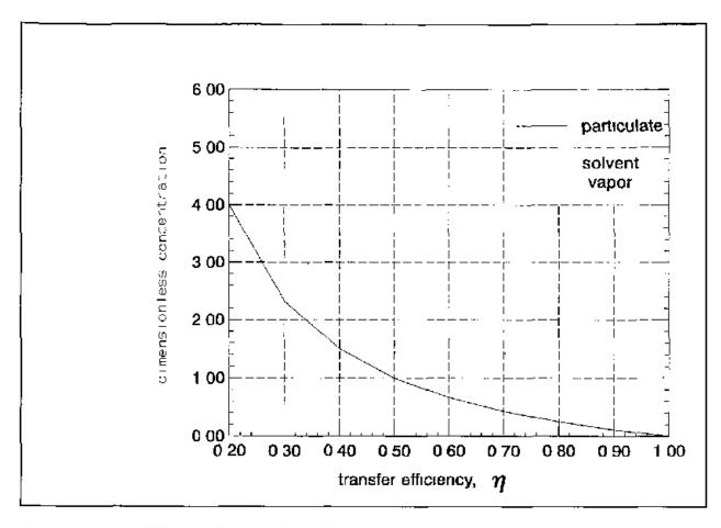
Figure 1 Effect of transfer efficiency upon particulate and vapor overspray concentrations assuming mixing in a spray painting booth
