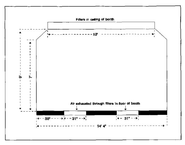
Figure 10 Cross section of spray painting booth during first set of tests
