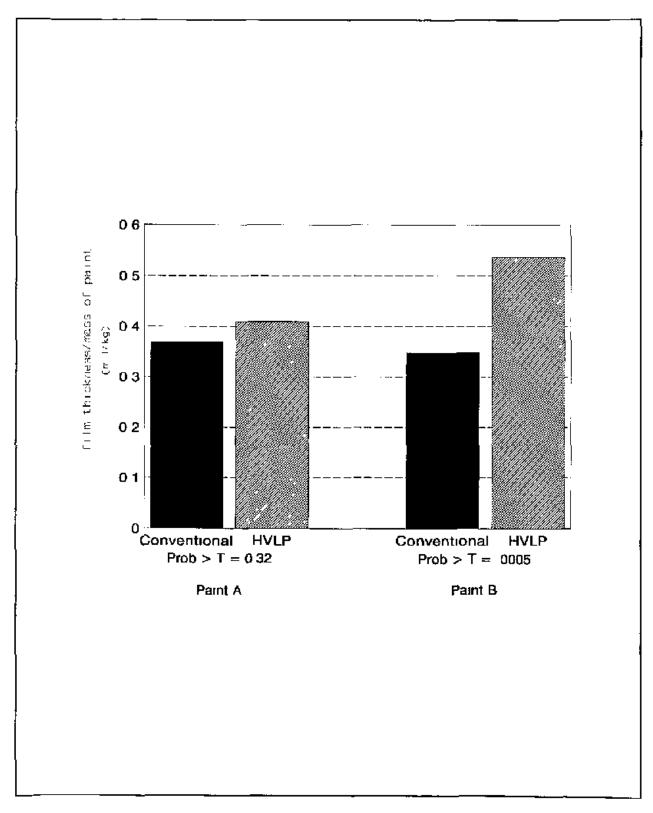
Figure 6 The effect of spray paint gun upon film thickness per mass of paint used varies with the paint tested
