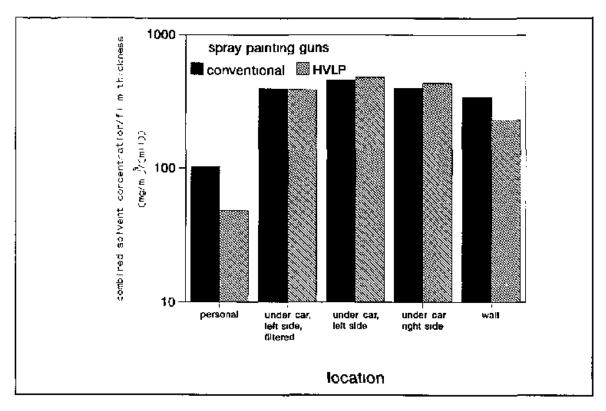
Figure 8 The effect of spray painting gun and location upon the geometric means of the combined solvent concentrations
