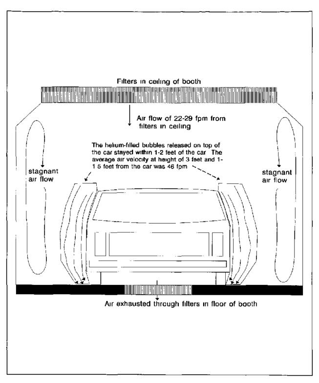
Figure 3 Schematic illustration of air flow patterns in booth. The air flow rates were deliberately reduced from the design specification of 10,000 cfm to an air flow between 5400 and 7100 cfm.
