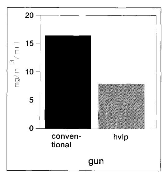
Figure 7 Effect of spray painting gun upon geometric mean particulate overspray concentration
