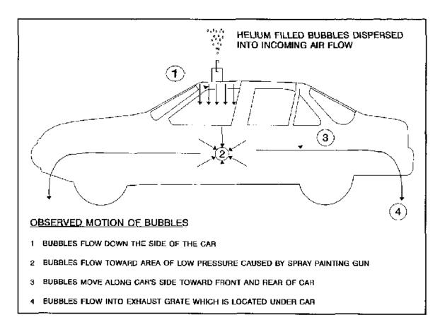
Figure 4 Motion of helium bubbles when the painter simulates painting side of car with empty spray painting guns
