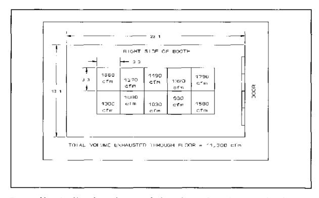
Figure 11 Airflow distribution of the exhaust from the paint booth
