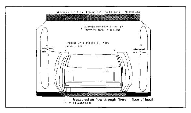
Figure 13 Smoke tube traces and exhaust volumes in the spray painting booth. The velocities around the car are shown in Figure 12
