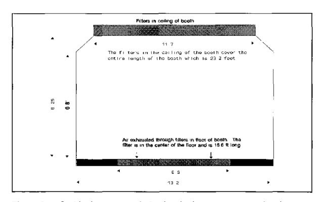
Figure 5 Inside dimensions of the downdraft spray painting booth
