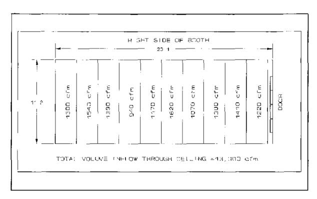
Figure 10 Airflow distribution into the paint booth
