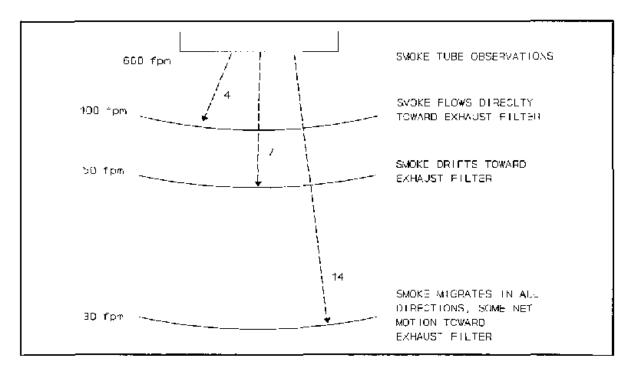
Figure 9 Air velocities and observations of smoke motion at the vehicle preparation station when air shower is not in use
