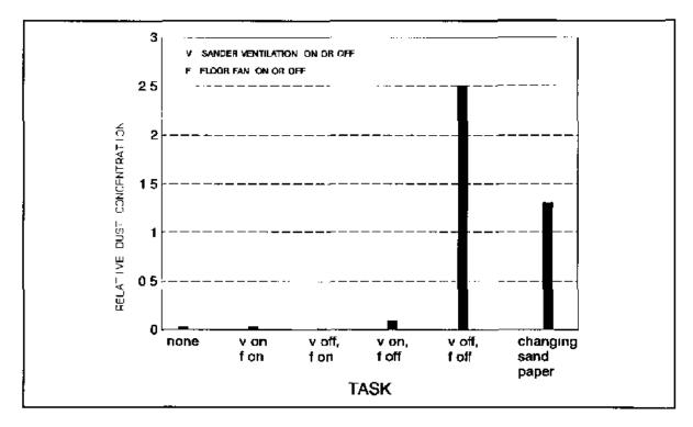
Figure 8 Relative dust concentration when worker is using orbital sander to smooth body filling compound on a car door
