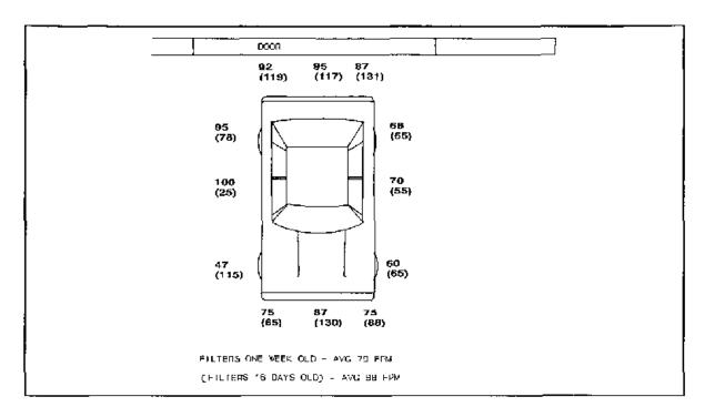
Figure 12 Air velocities around a car on two different days during the study. These velocity measurements were taken at a height of 3 feet and a distance of 1.5 feet from the car
