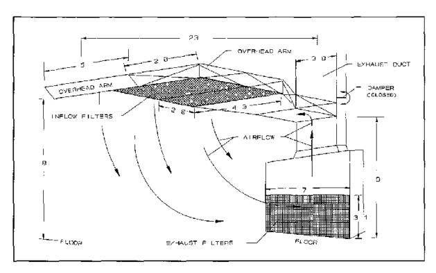
Figure 2 Vehicle preparation station and its airflow patterns while operating in the "recycle mode"
