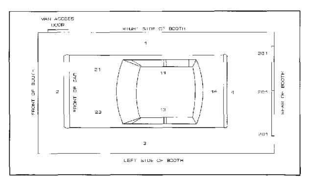
Figure 14 The areas of the car being painted (for example, Area 3 is the left side of the car)
