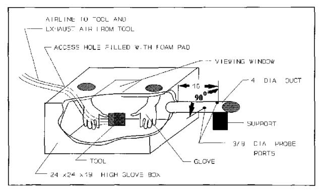
Figure 6 Apparatus for measuring air volumes through ventilated sanders NOTE The air flows into this box through the 4" diameter duct
