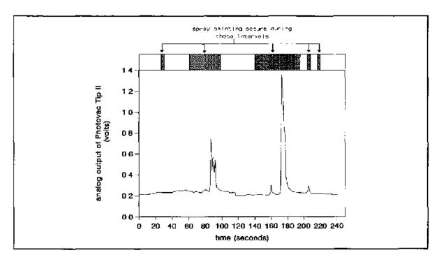
Figure 15 Relative concentration while gravity feed gun was used to apply clear coat to the side of car (run 4) The ventilation does not always keep overspray away from the worker's head
