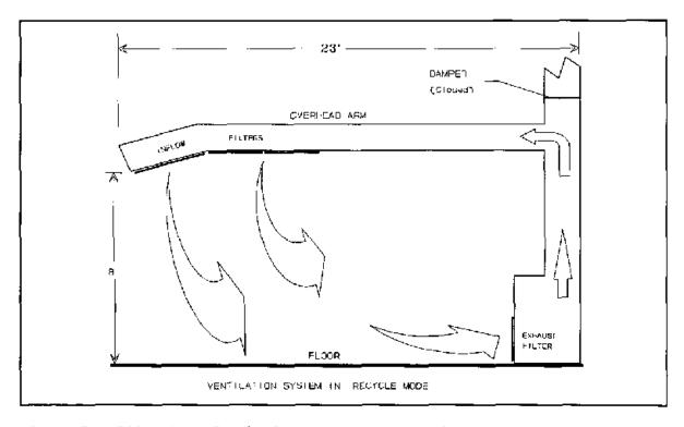
Figure 3 Side view of vehicle preparation station
