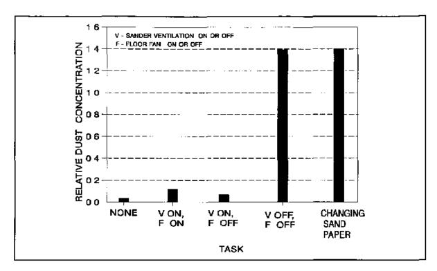
Figure 7 Relative dust concentration when in-line sander is used to smooth body filling compound on the side of a car door
