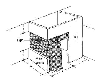
Figure 6 Diagram of the rinse booth installed before survey 4
