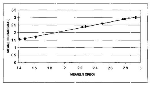
Figure 15 Mean Ln(charcoal) versus Mean Ln(ORBO) for Stripping in Survey 3 & 4 Fitted Equation LN(charcoal)=0 135 + 0 989, R<sup>2</sup>=0 987 Note Run 5 in Survey 4 and Run 1 in Survey 3 excluded
