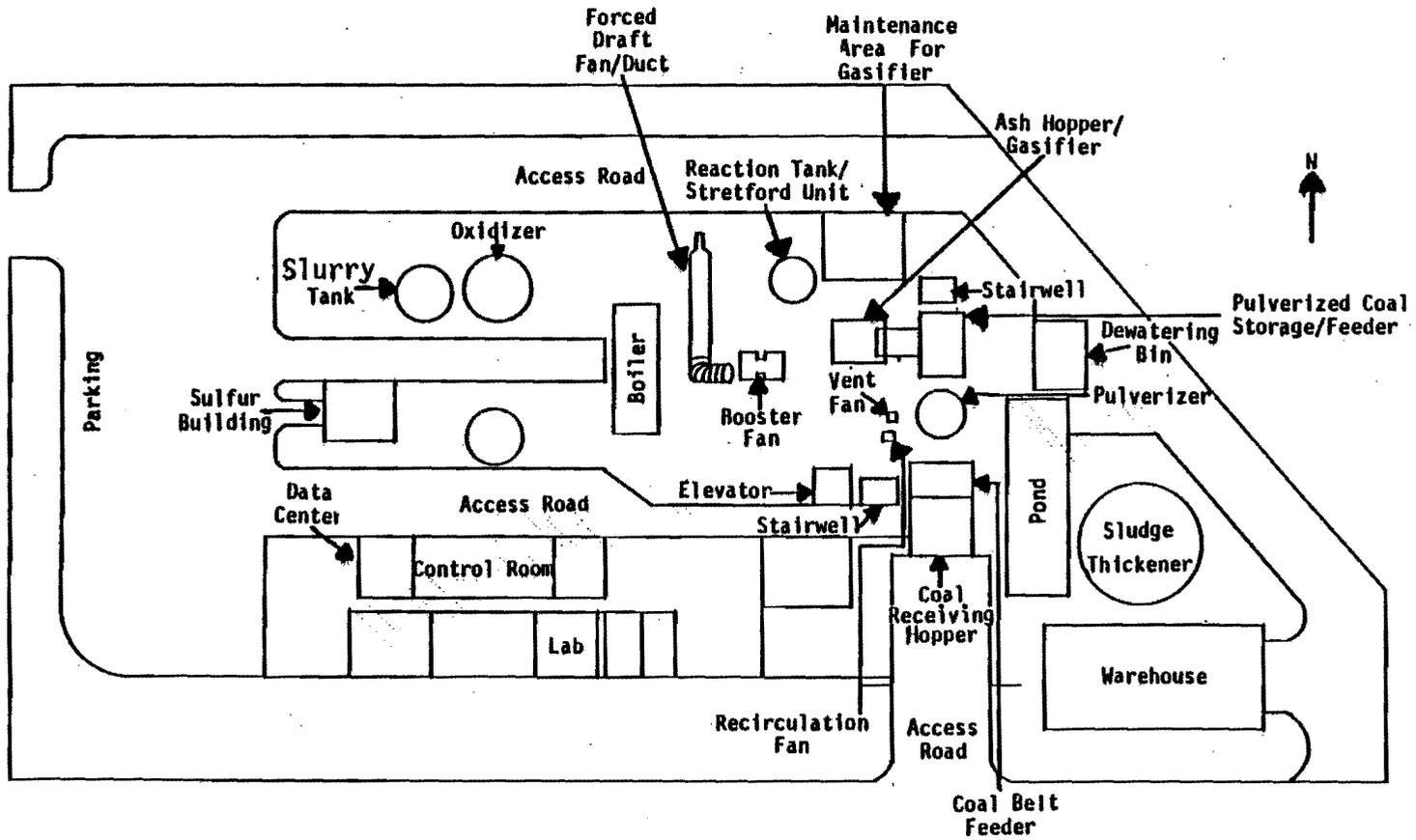
Figure 1. Layout of the Combustion Engineering Process Demonstration Unit
