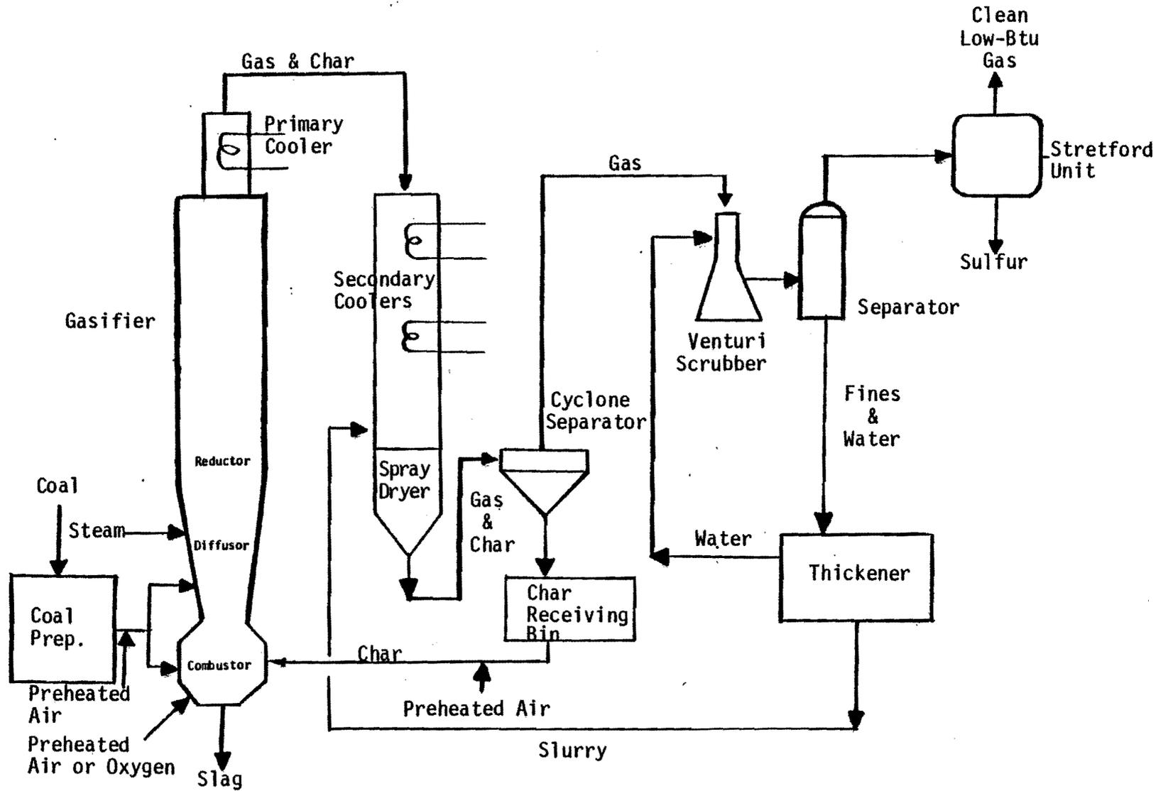
Figure 2. Schematic of the Combustion Engineering Low-Btu Coal Gasification Process
