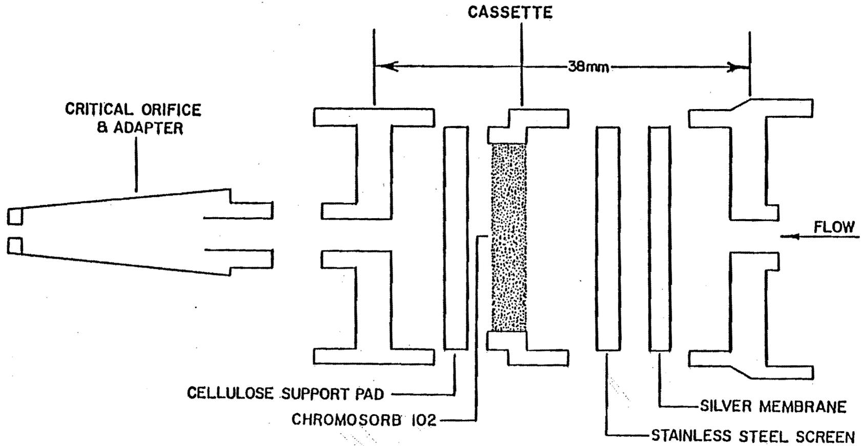
Figure A-1. HIGH-VOLUME SAMPLING DEVICE FOR PNA
