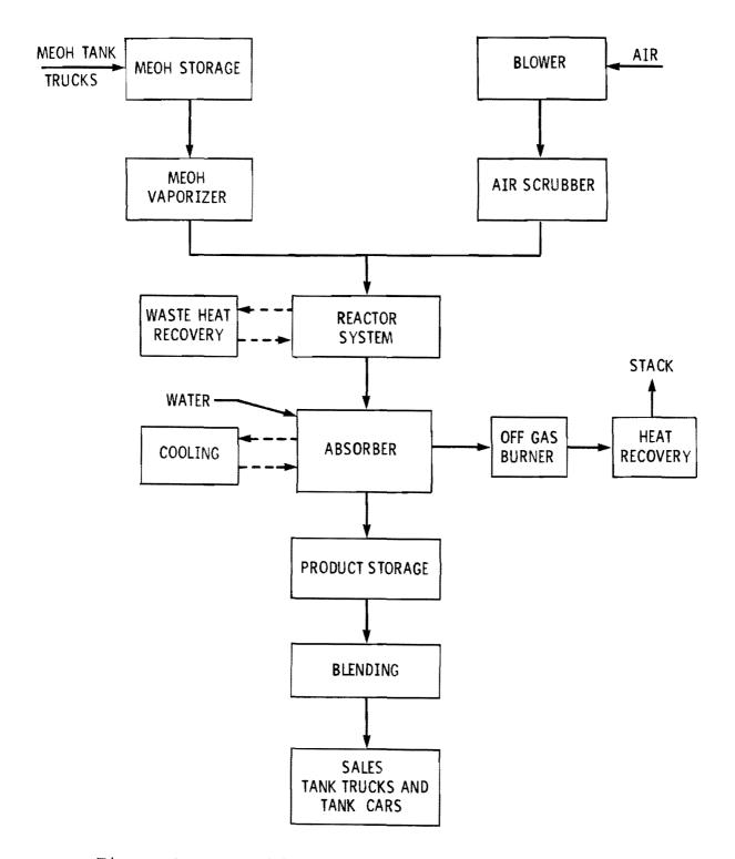
Figure 2. Formaldehyde process - block flow diagram.
