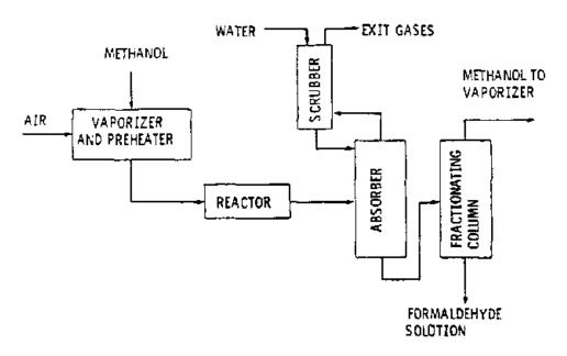
Figure 3. Formaldehyde production process using a silver catalyst [21].
