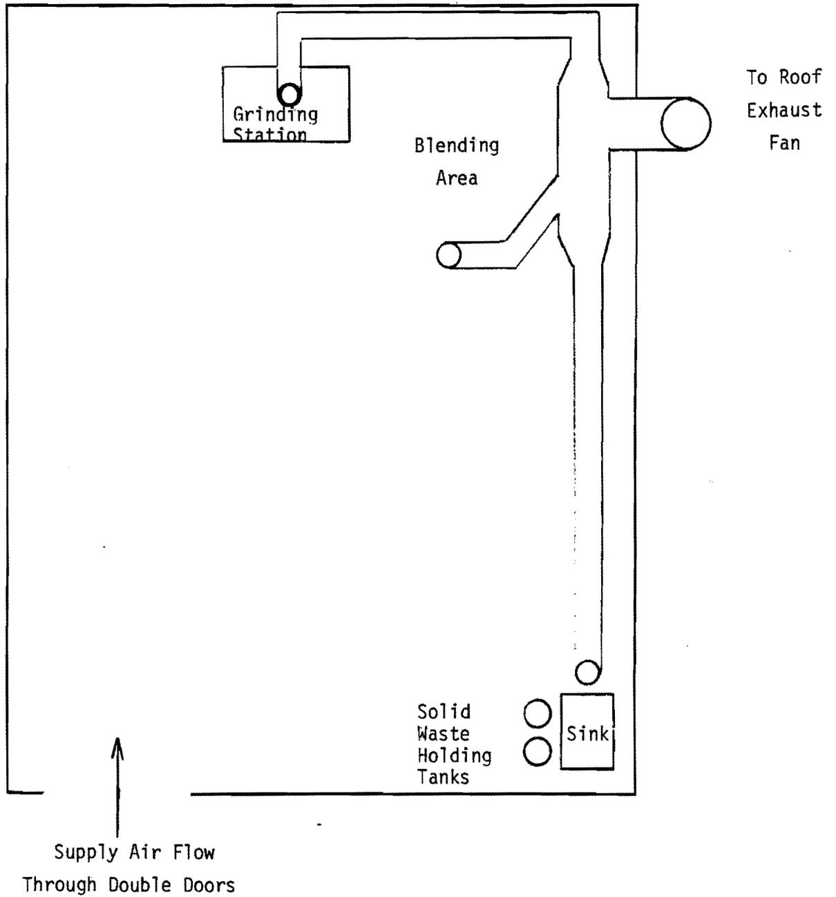
Figure 2. Gel Room Ventilation System
