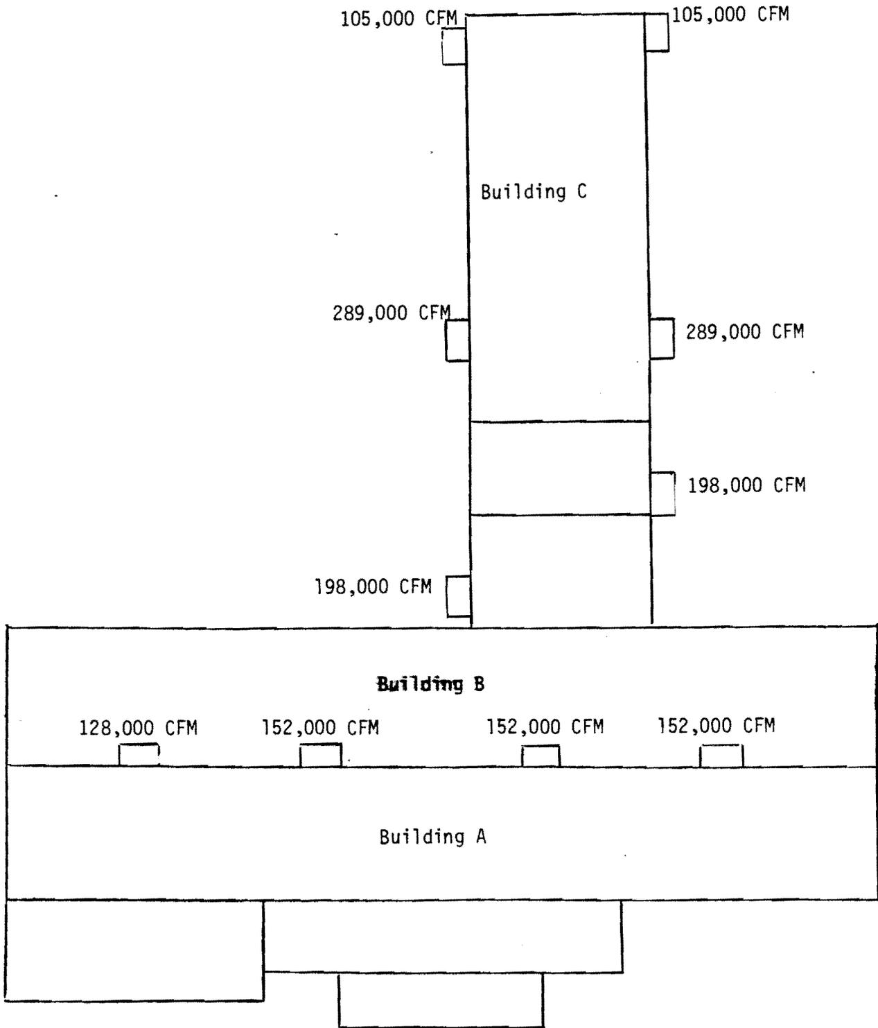
Figure 2: Plant Layout Showing Air Supply System Intakes.
