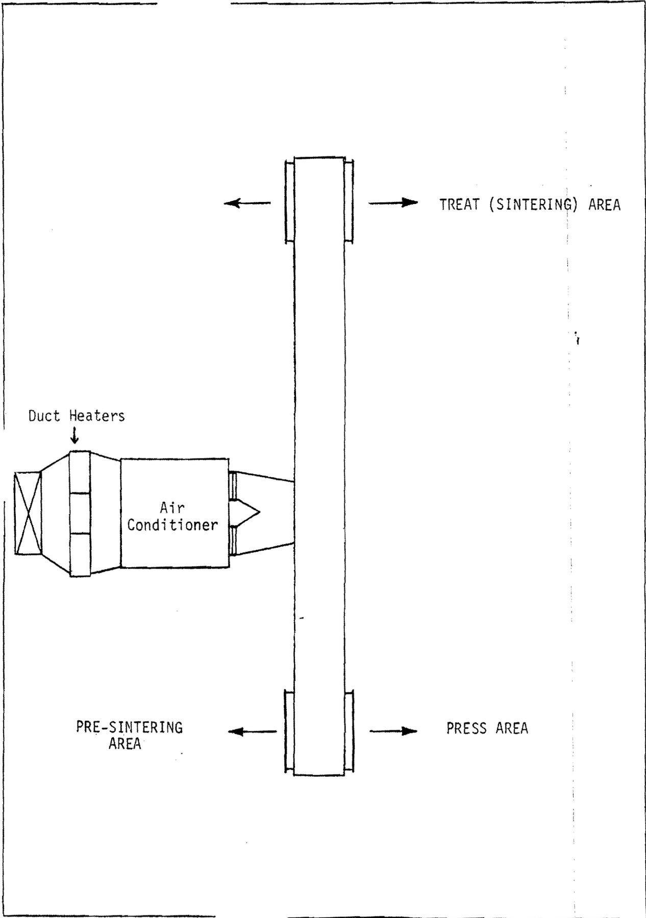
Figure 1. Press and Treat Room - Air Supply System.
